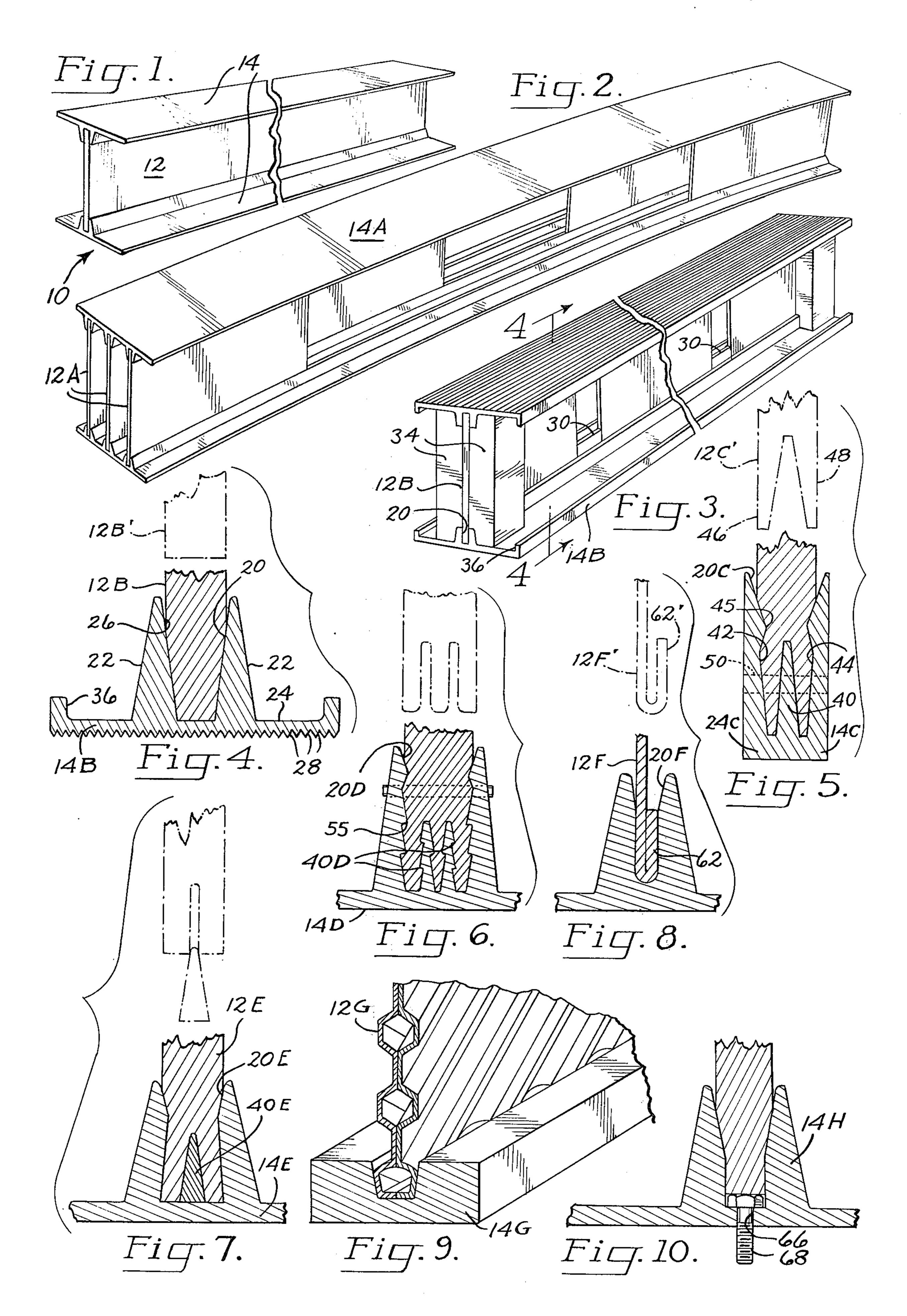
flange element has a channel receiving an edge margin of the web.
