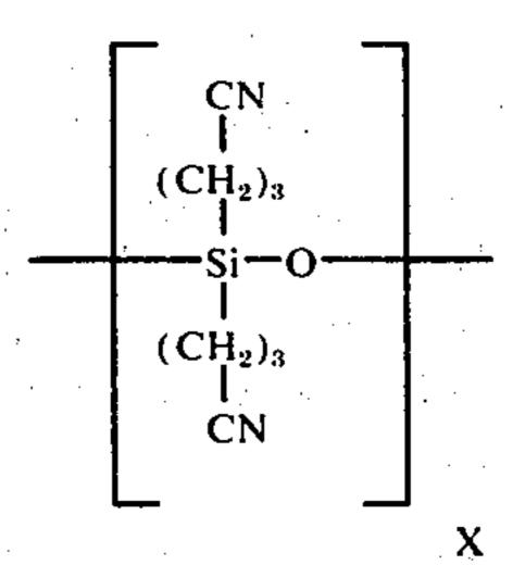
Where X is a whole number between 5 and 20. This polymer material is a di(cyanopropyl) substituted silicone.
