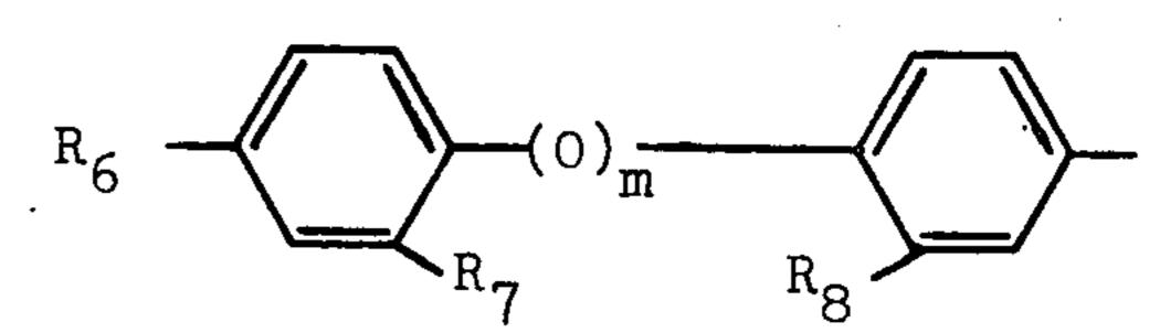
in which m is 0 or 1, and  $R_6$ ,  $R_7$  and  $R_8$  may be the same or different and are selected from hydrogen, chlorine or fluorine, at least one being chlorine or fluorine.
