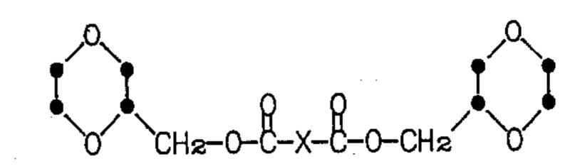
wherein X is an acrylic or cyclic aliphatic or aromatic moiety having from 1 to 8 carbon atoms are produced by esterification of 1,4-dioxanemethanol with a dicarboxylic acid of 3 to 10 carbon atoms or a corresponding acid anhydride. The novel esters are useful as plasticizers, viscosity improvers, and in waxes and polishes.
