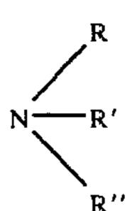
where R is lower alkyl or hydroxy-substituted lower alkyl and R' and R' are hydrogen or R, and the temperature of said aqueous diluent being between 75° and 100°C., (c) agitating the aqueous mixture at 75° to 100°C. to form a pigment slurry, and (d) recovering the metal phthalocyanine pigment from the slurry.
