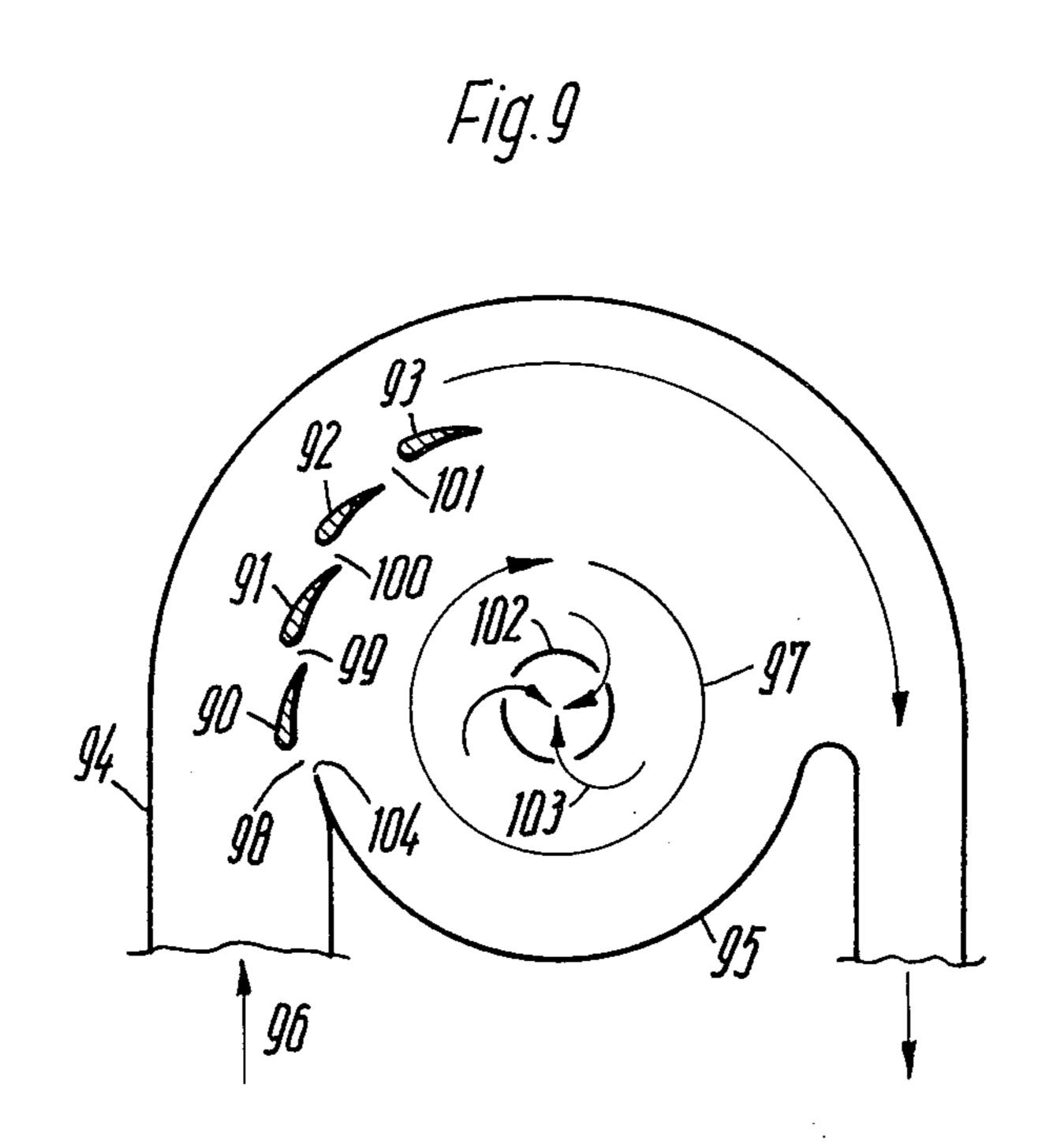
METHOD AND APPARATUS FOR SEPARATING SUSPENDED MATTER FROM A FLUID BY CENTRIFUGAL FORCE
