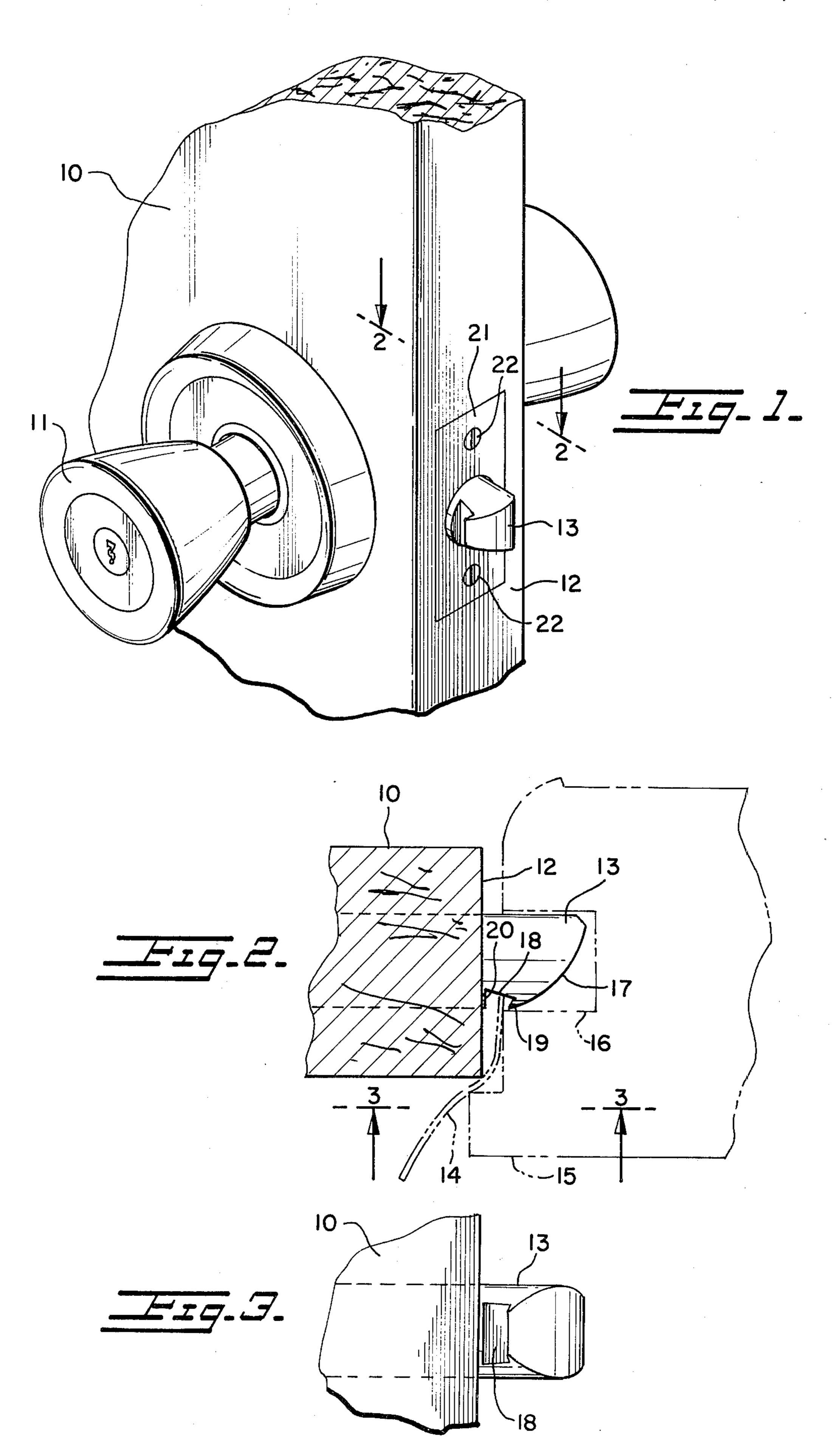
This invention relates to an improved latch bolt for a door lock which prevents unauthorized entry.
