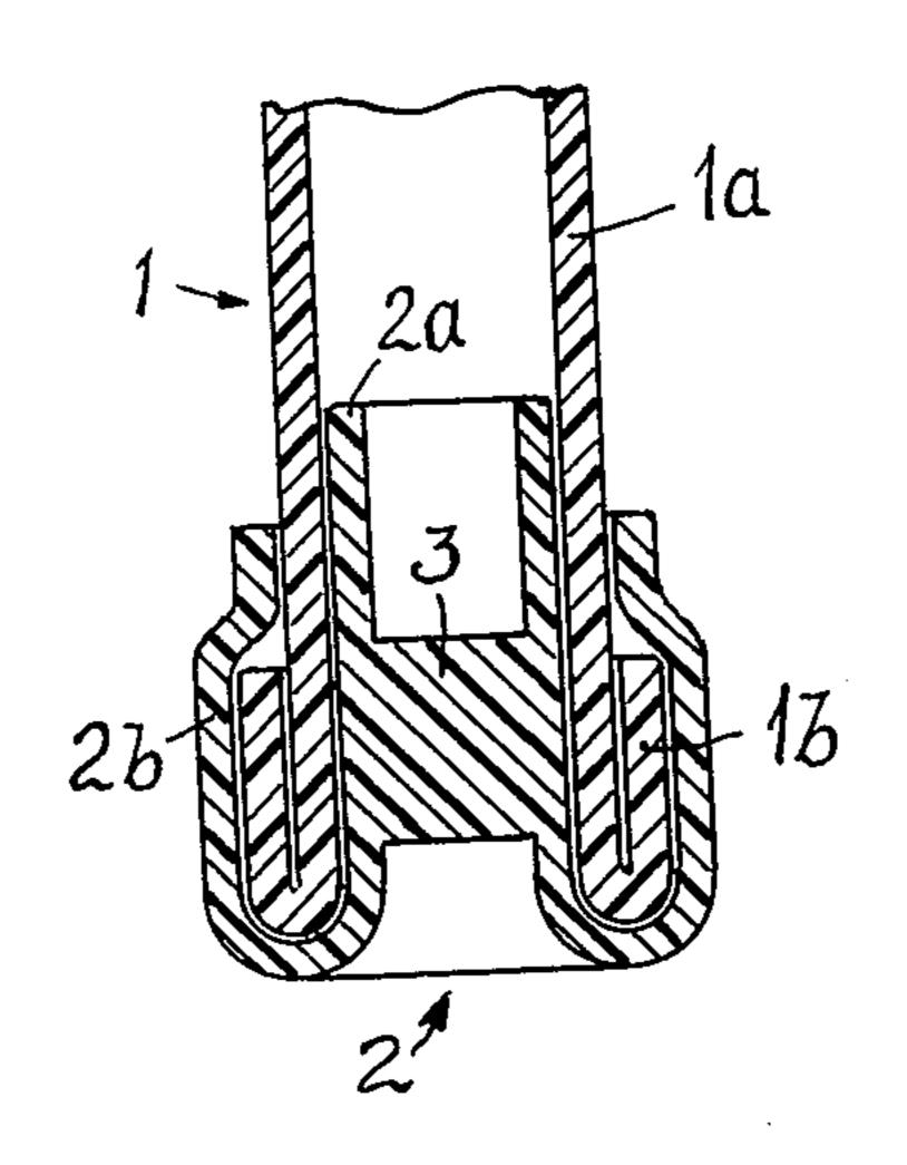
MEANS FOR CONNECTING AN ELASTOMERIC TUBING TO A MEMBER
