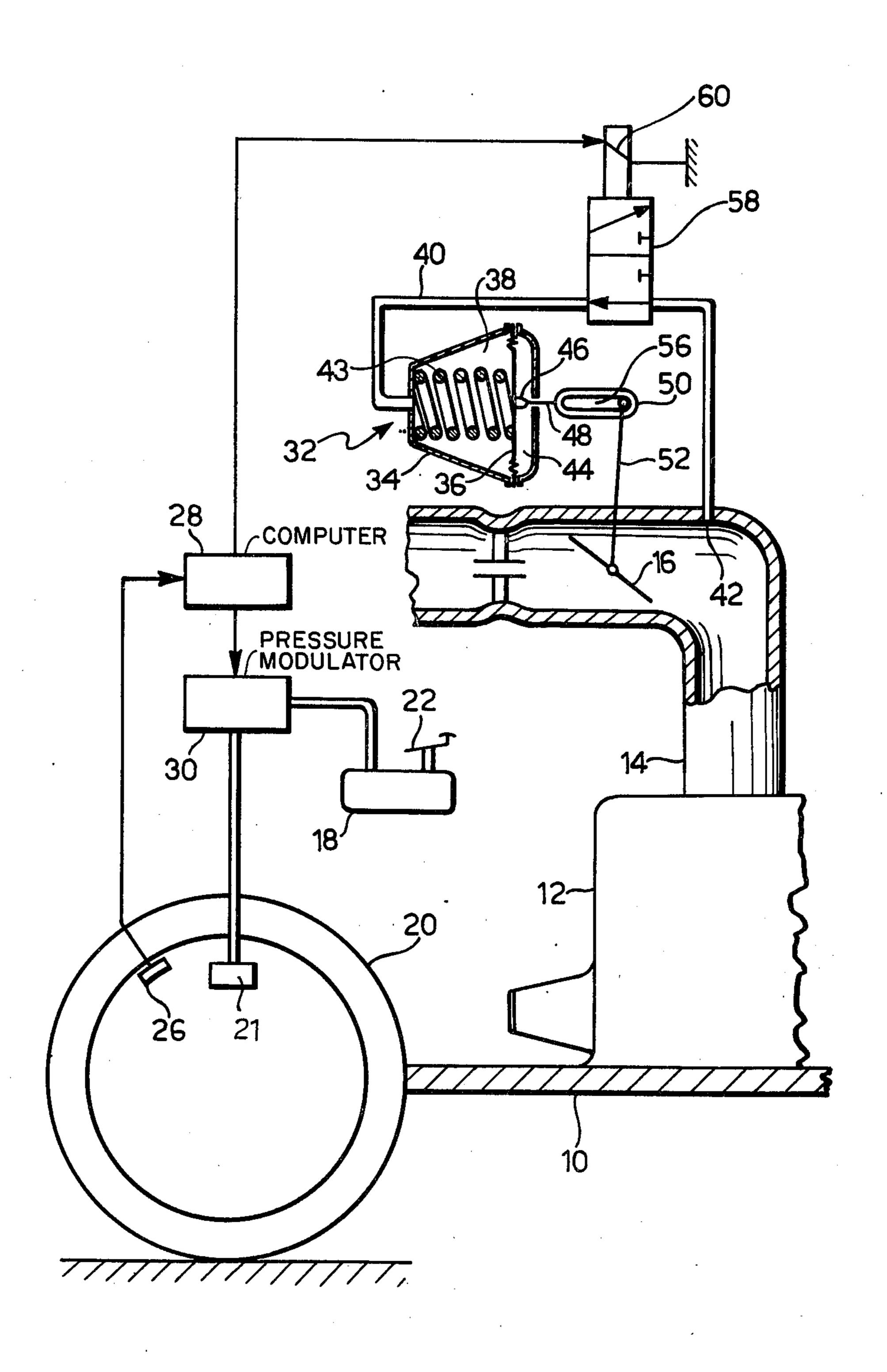
brake fluid in the brake actuator 21 in the event of incipient skidding of the wheel.
