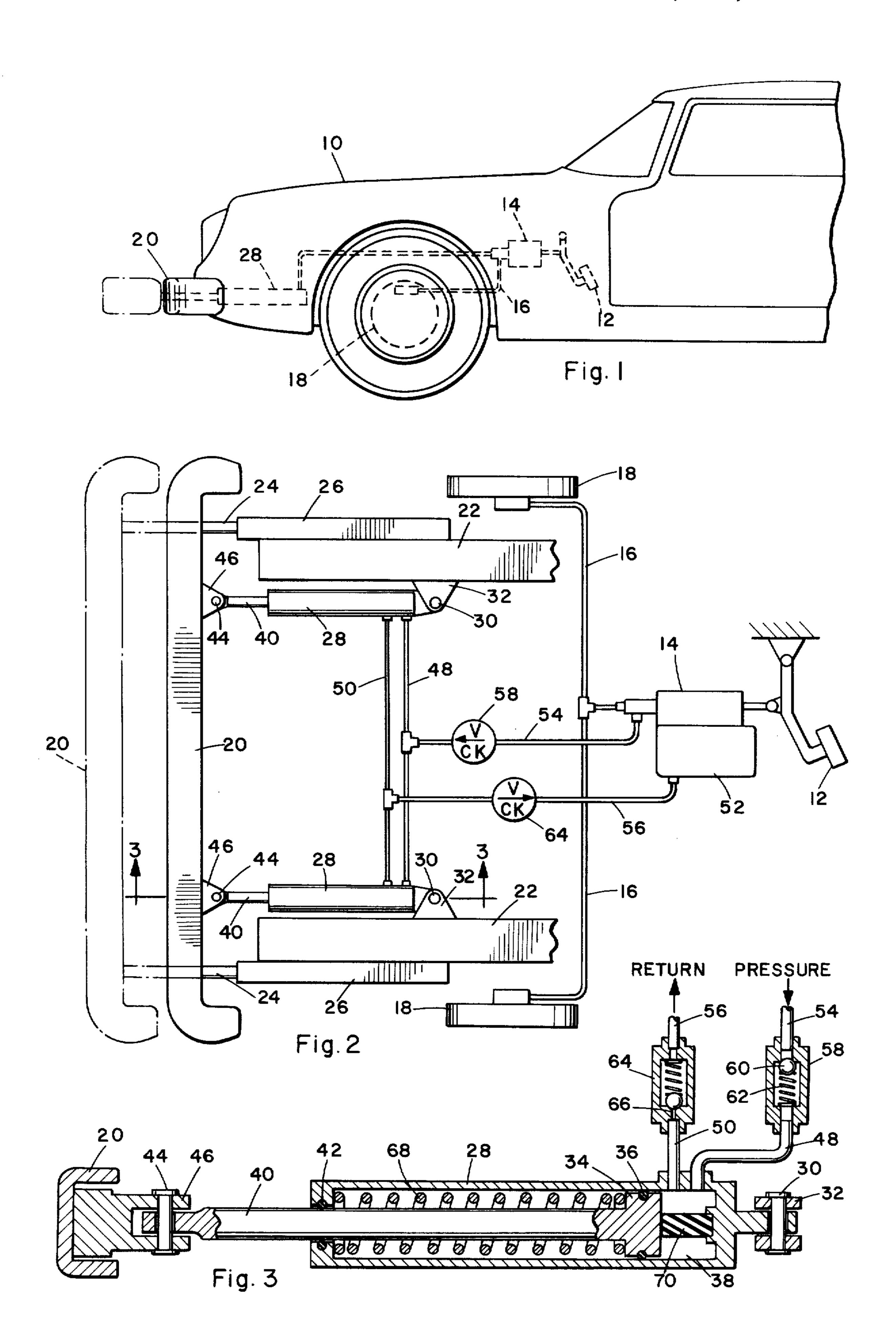
forward and reverse sliding motion between the bumper bar and frame, such as the bars 24 which are slideably received in the elongated sockets 26 which are welded or otherwise attached to the frame members.
