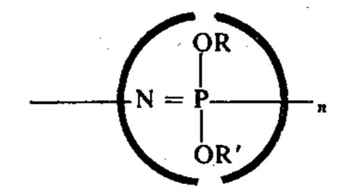
where R and R' are the same or different alkyl or alkenyl radicals having from one to six carbon atoms and n is an integer of at least 3 and not more than about 20. 20 These fibers are prepared by incorporating a flameretardant amount of the phosphonitrilic polymer into filament-forming viscose, and spinning and regenerating the filament.
