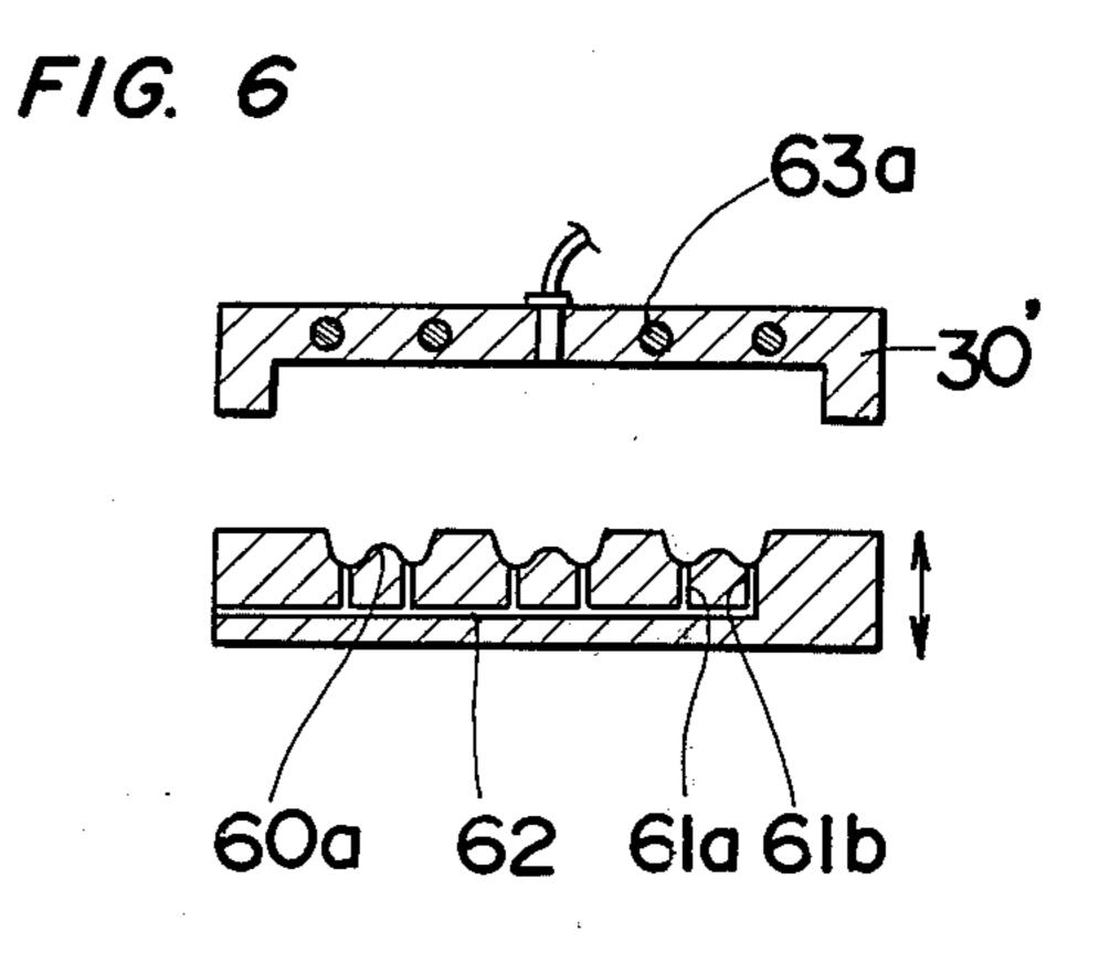
MOLD ASSEMBLY FOR USE IN PACKAGING MACHINE
