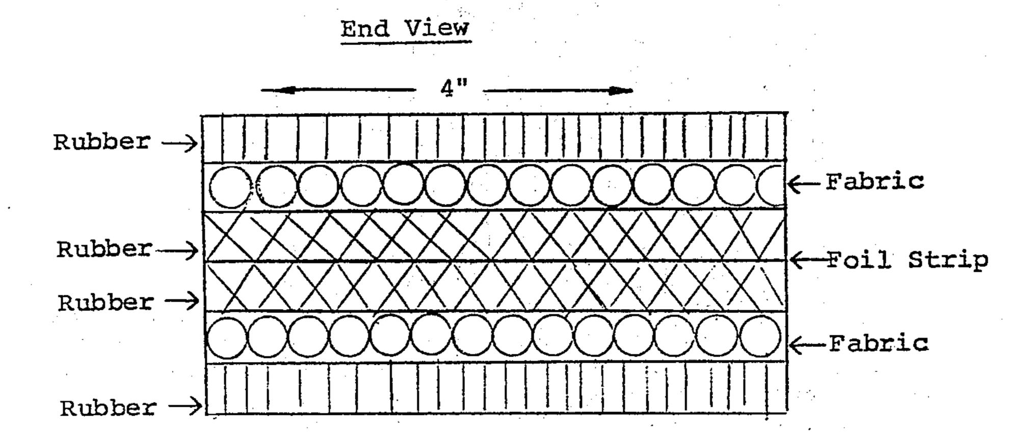
2. The test cord is wound onto the drum at 20 ends per inch to obtain a 5 inch width. 3. This rubberized fabric is used to fabricate specimens having the composition shown in the following sketch:
