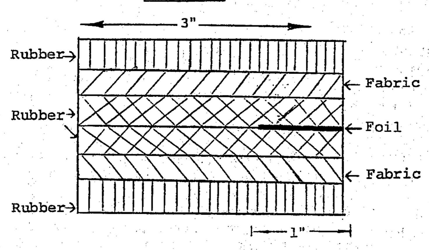
4. This "sandwich" is cured in a mold for 6 minutes at a pressure of 4 tons and a temperature of 350° F.
