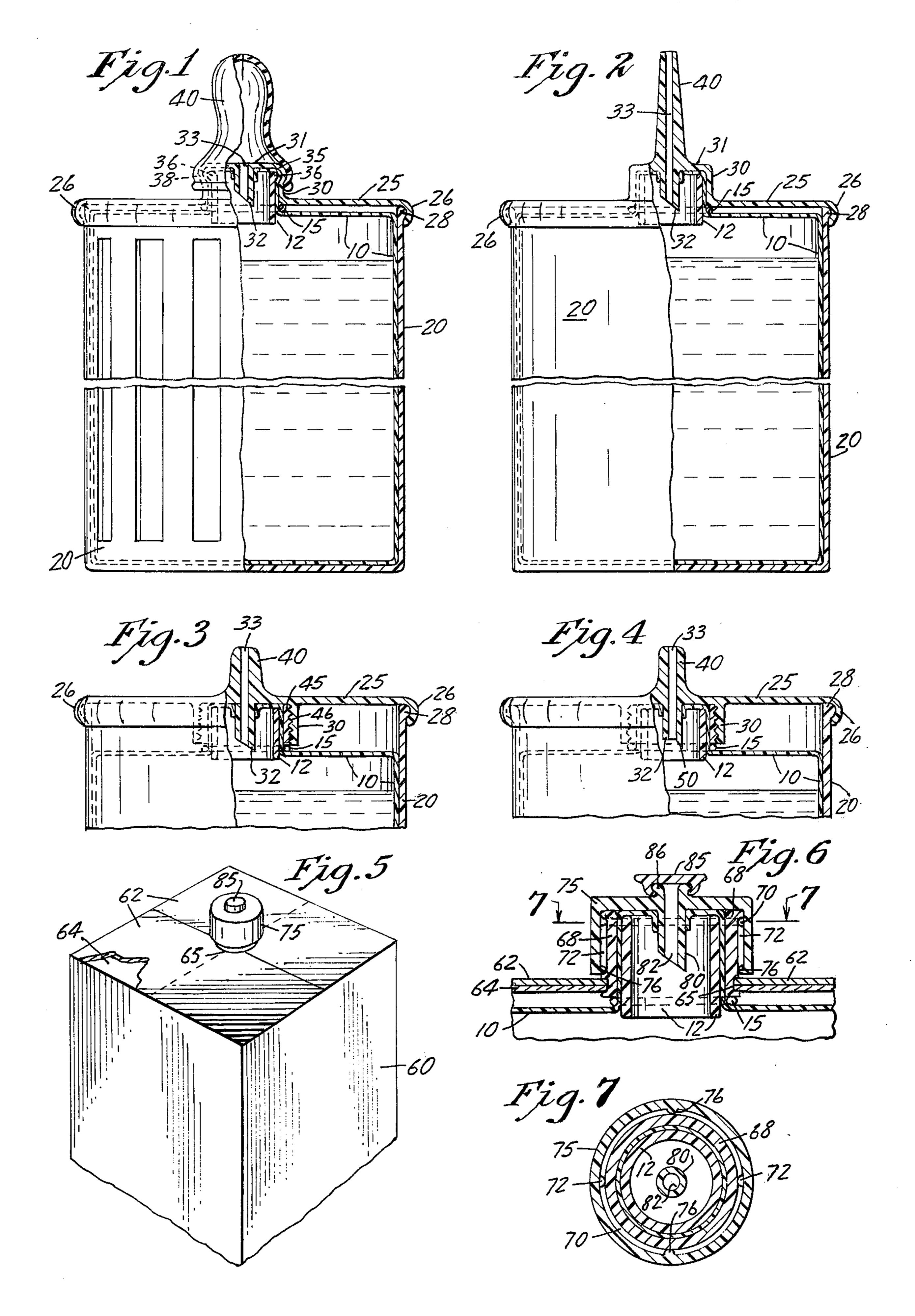
It is therefore the general object of this invention to provide an improved and inexpensive means for packaging and dispensing fluids such as liquids contained in a flexible walled sealed fluid-container pouch having a rigid tubular element positioned in a wall thereof.
