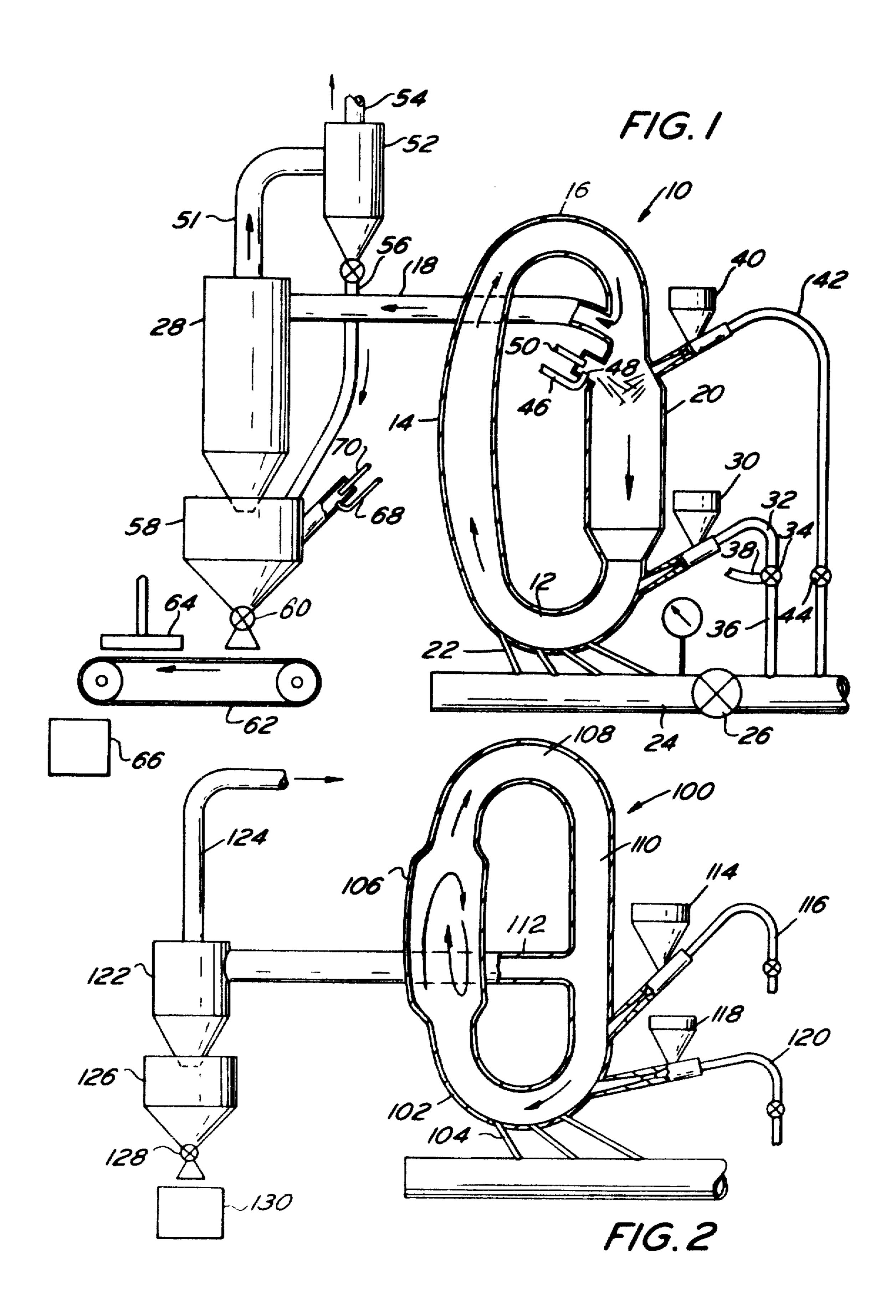
APPARATUS FOR MIXING PULVERIZING AND GRINDING BLACK POWDER
