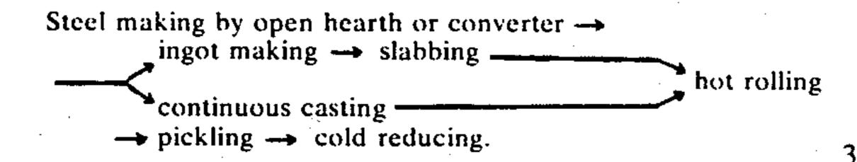
In the hot rolling stage, finishing at and coiling at a low temperature is preferred, because the coiling at a low temperature is more advantageous than that of high temperature for obtaining the strength required. 40 The strip is then subjected to either of the following three types of continuous annealing, which is another important requirement in this invention.
