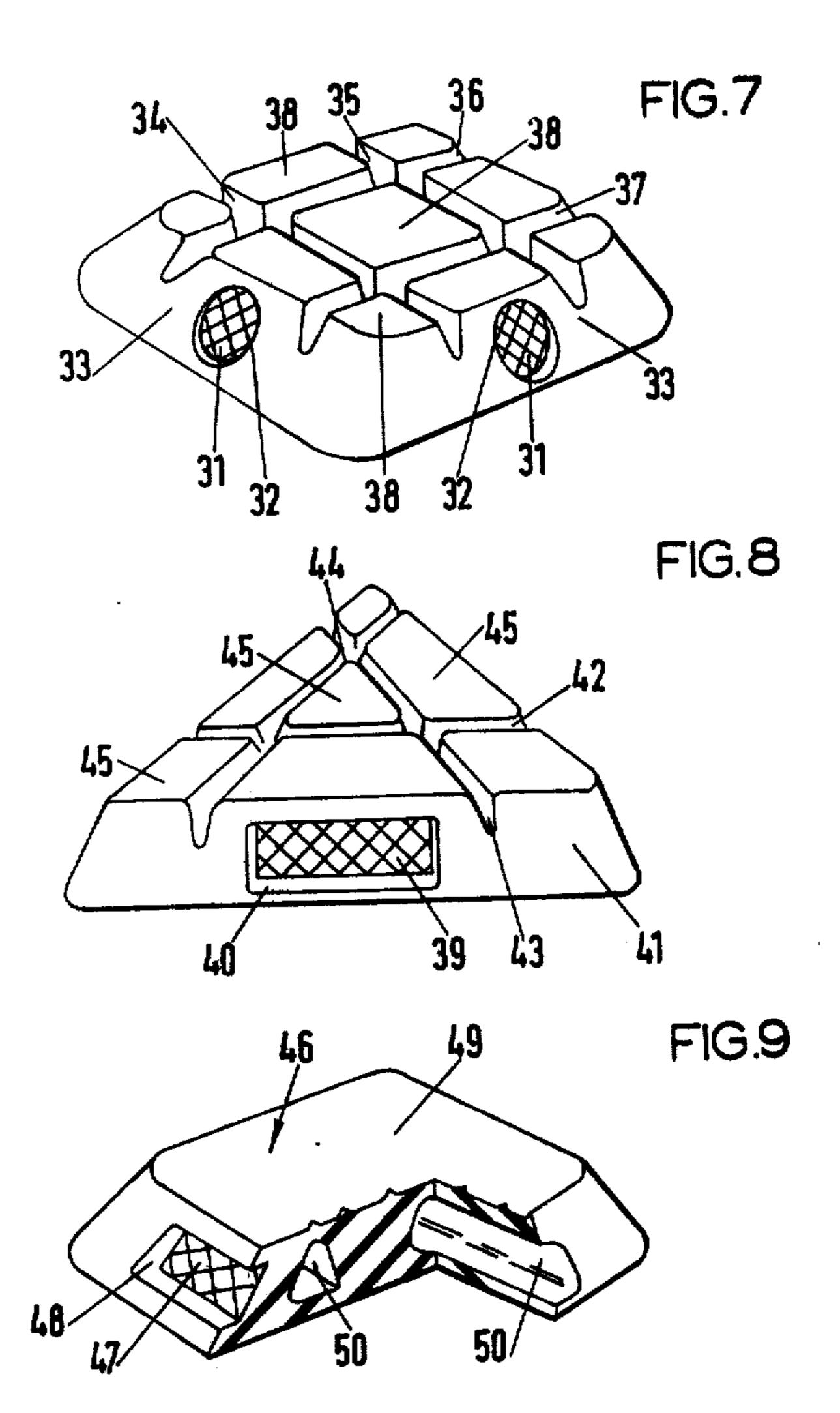
This invention relates to reflector studs. It is particularly concerned with housings for reflective devices and sepecially to reflective road marker studs such as may be used to indicate traffic lanes. Thus the invention is particularly concerned with a road marker stud adapted to accommodate static and dynamic pressures imposed by vehicle wheels without detriment to its 10 reflective ability.
