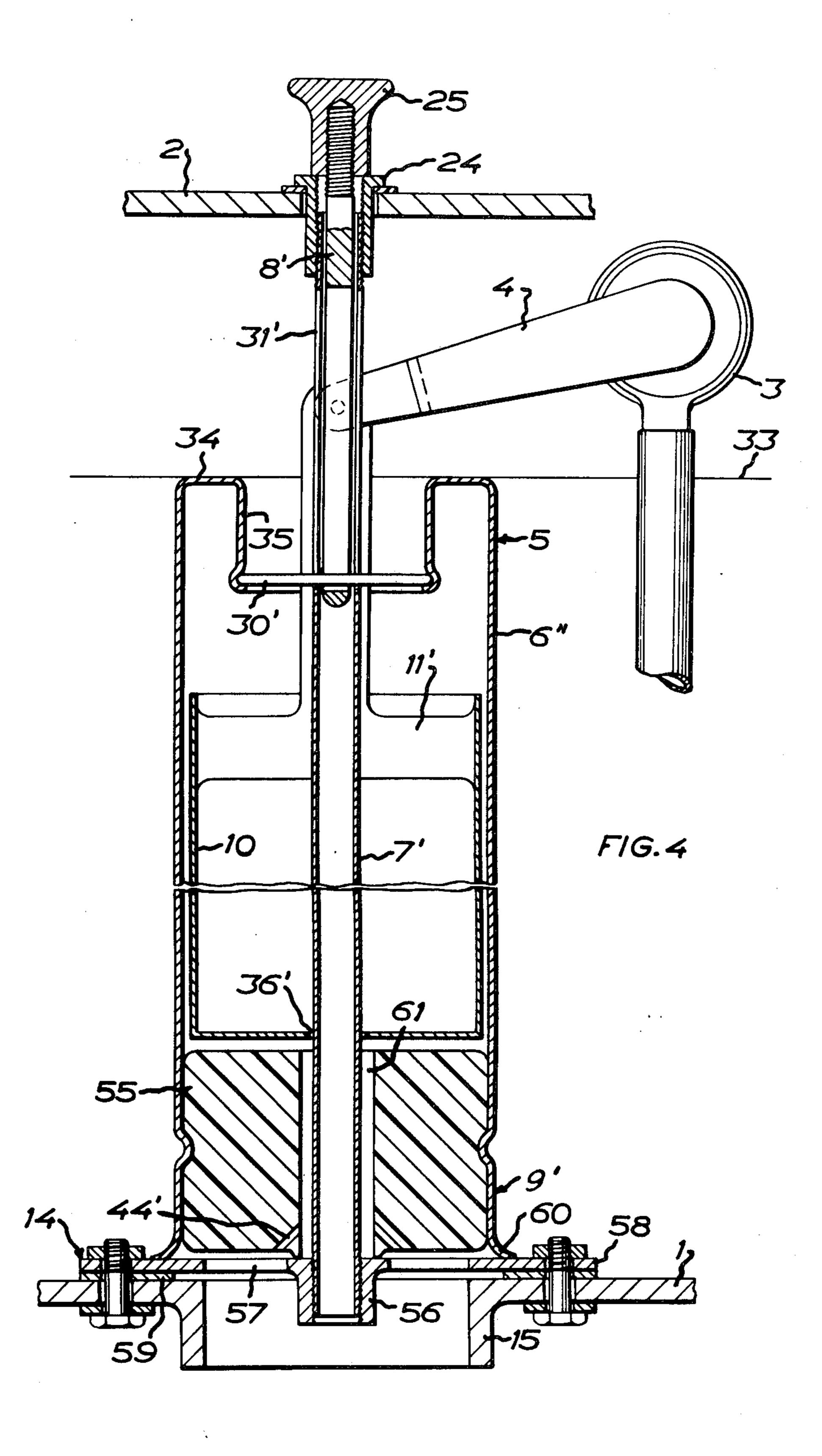
This invention relates to a flushing cistern, especially for water closets, comprising a container connected to a conduit for water under pressure via a refilling valve, an overflow, an outlet closable by means of a flushing valve, and a lift stem, adapted to open the flushing valve.
