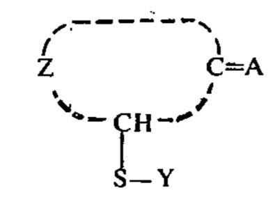
in which Z stands for a group of non-metallic atoms necessary for forming a carbon ring nucleus or heterocyclic ring nucleus, Y stands for a group capable of forming, on cleavage of the thioether linkage, a mercaptan type compound having development inhibiting activity together with the sulfur atom, and A stands for an oxygen atom or the group =NR in which R stands for a hydroxyl group or a amino group which may be substituted.
