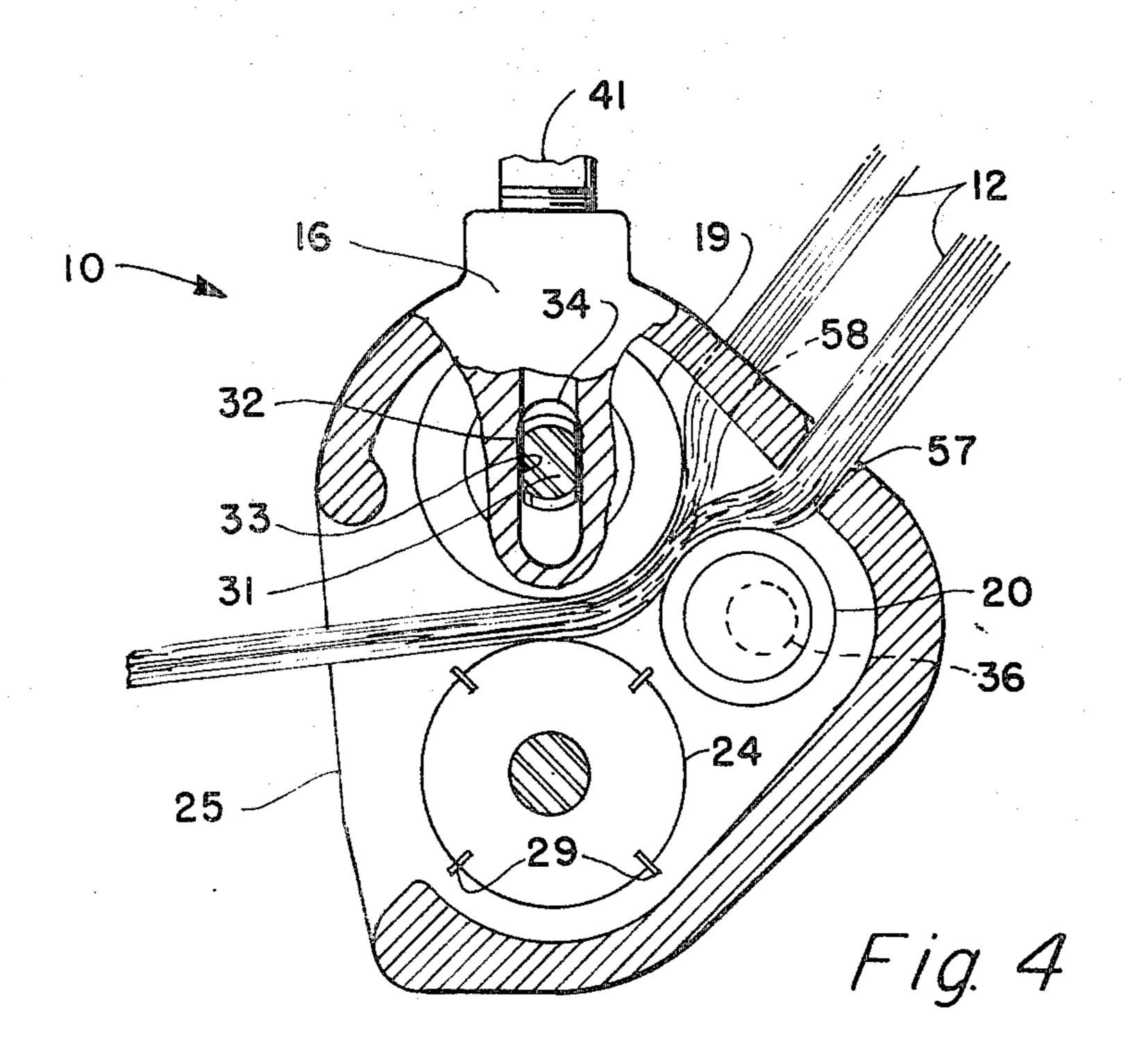
other is illustrated in United States Letters Pat. No. 2,787,314. The blades of the cutter roller press the glass roving against the back-up roller to thereby sever the roving into short lengths called "chop." The glass chop is ejected from the roving cutter into resin. A cutter roller typically operates at speeds of up to about 3,000 revolutions per minute.
