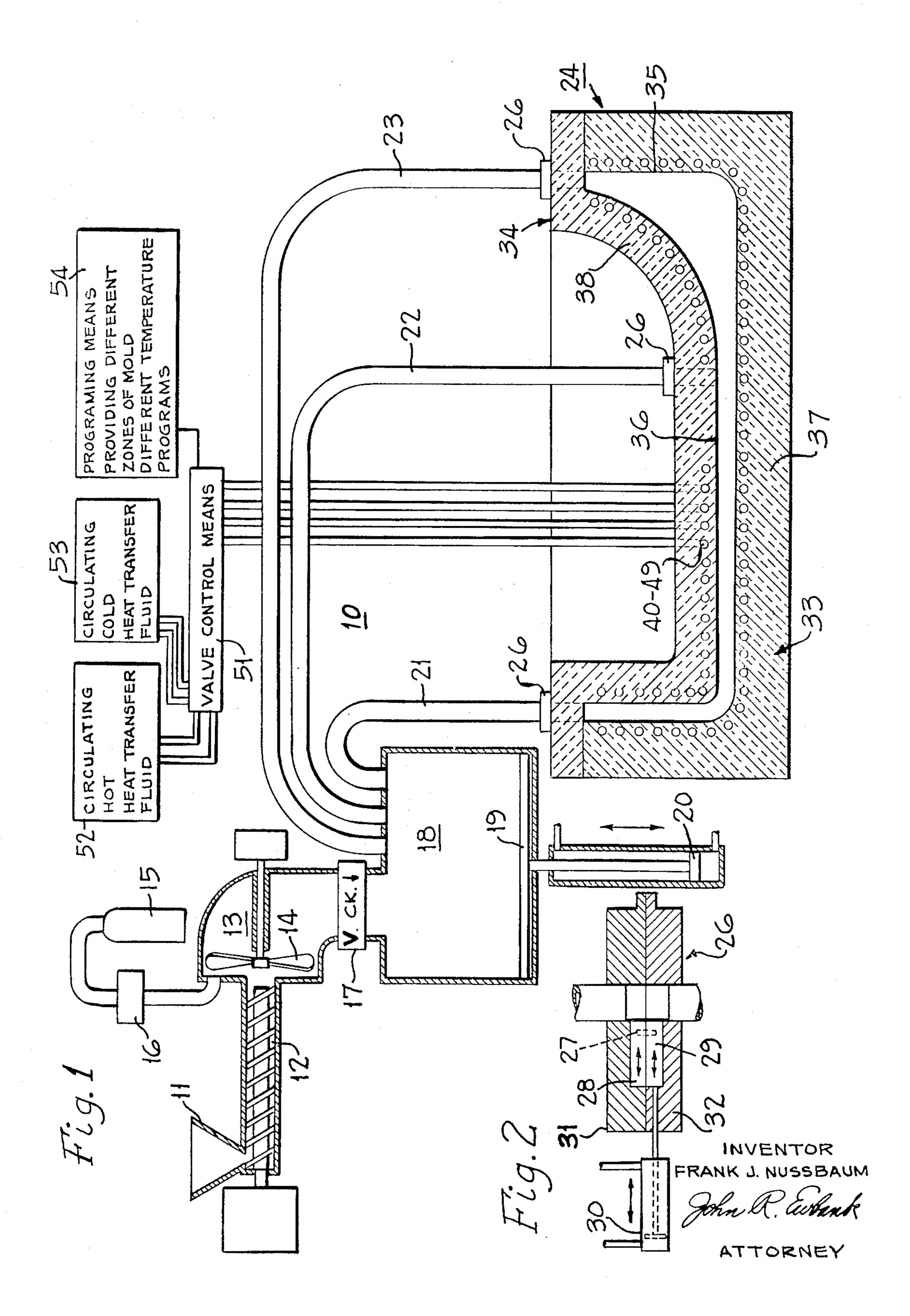
PROCESS OF MOLDING GIANT ARTICLES OF STRUCTURED PLASTIC
