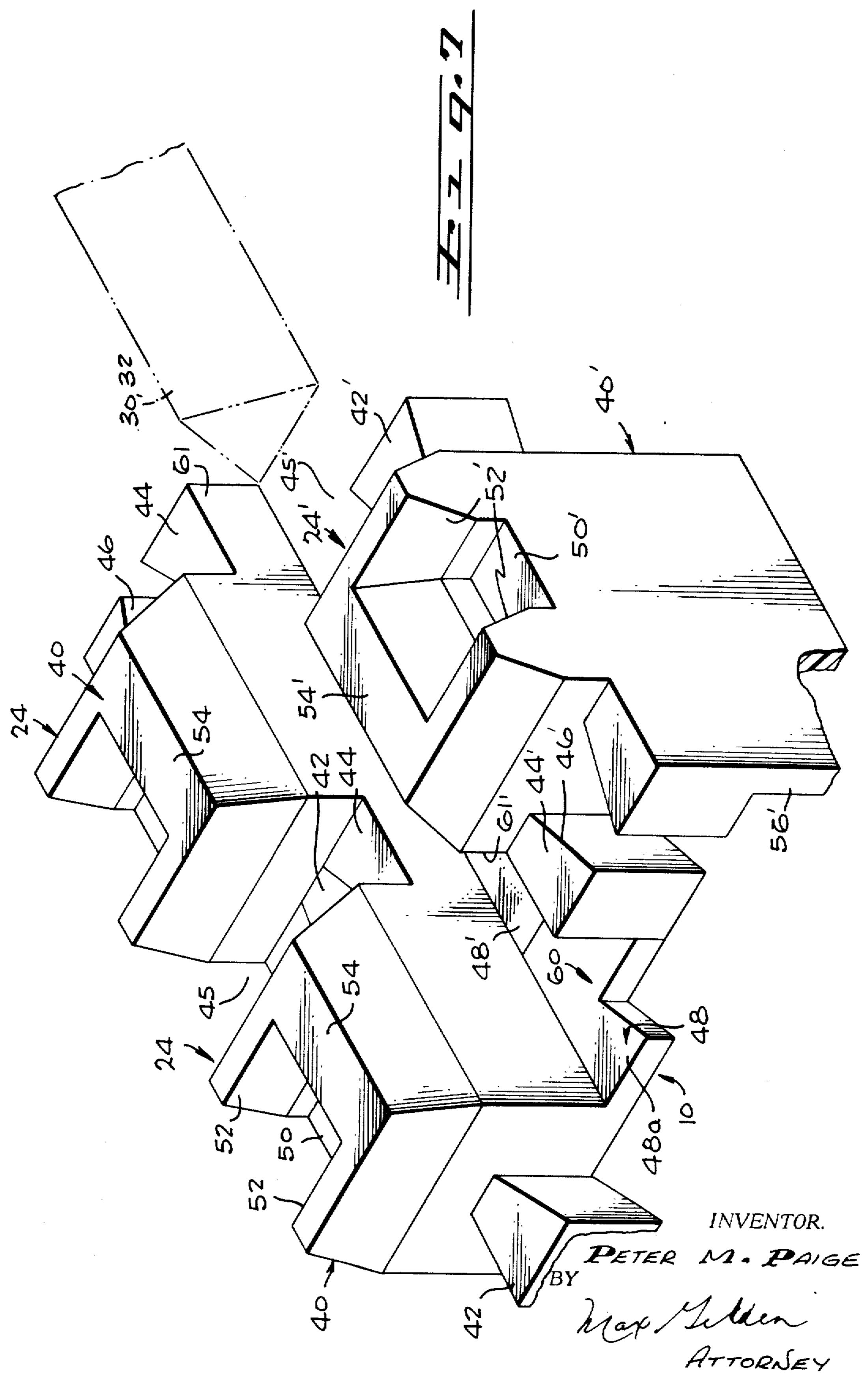
3,697,404 APPARATUS TO SUPPORT THE ELECTRODES AND BUS BARS IN AN ELECTROLYTIC CELL Peter M. Paige, 1200 N. Flores, Los Angeles, Calif. 90069 Filed Jan. 29, 1971, Ser. No. 110,943 Int. Cl. C23b 5/70
