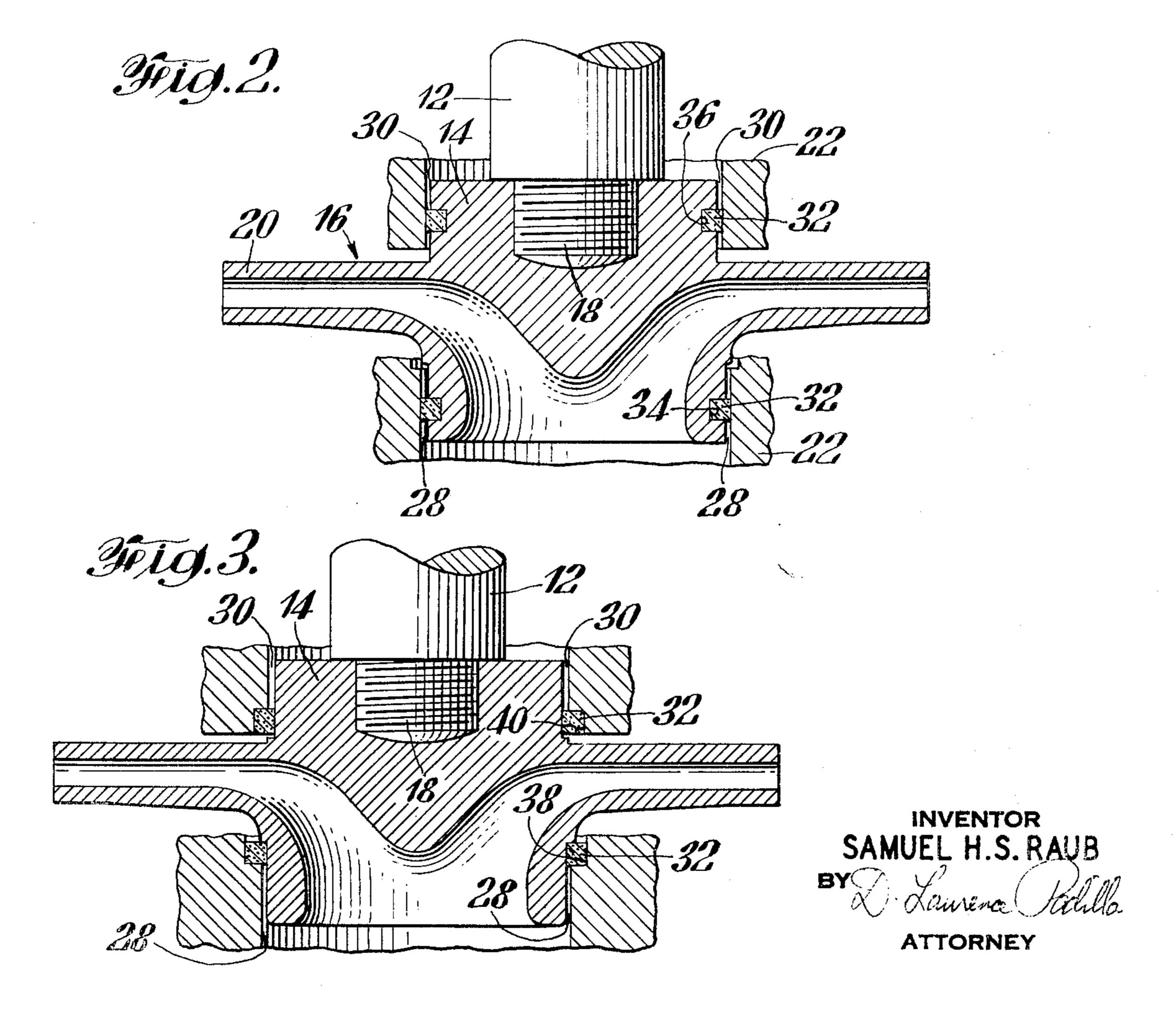
INTERNAL SEALS FOR PUMPS WITH ENCLOSED IMPELLERS
