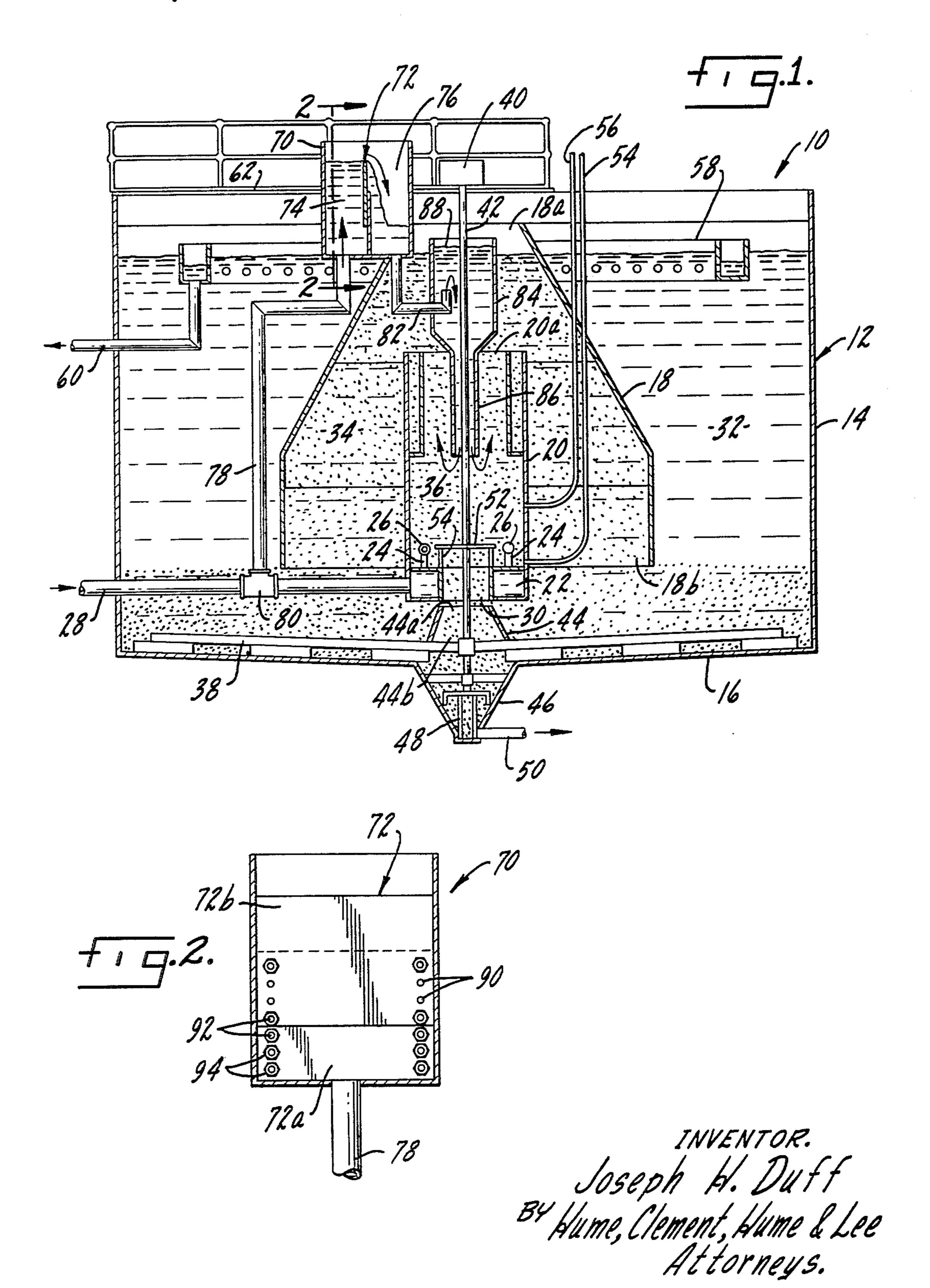
FLOW CONTROL MEANS FOR WATER TREATING APPARATUS
