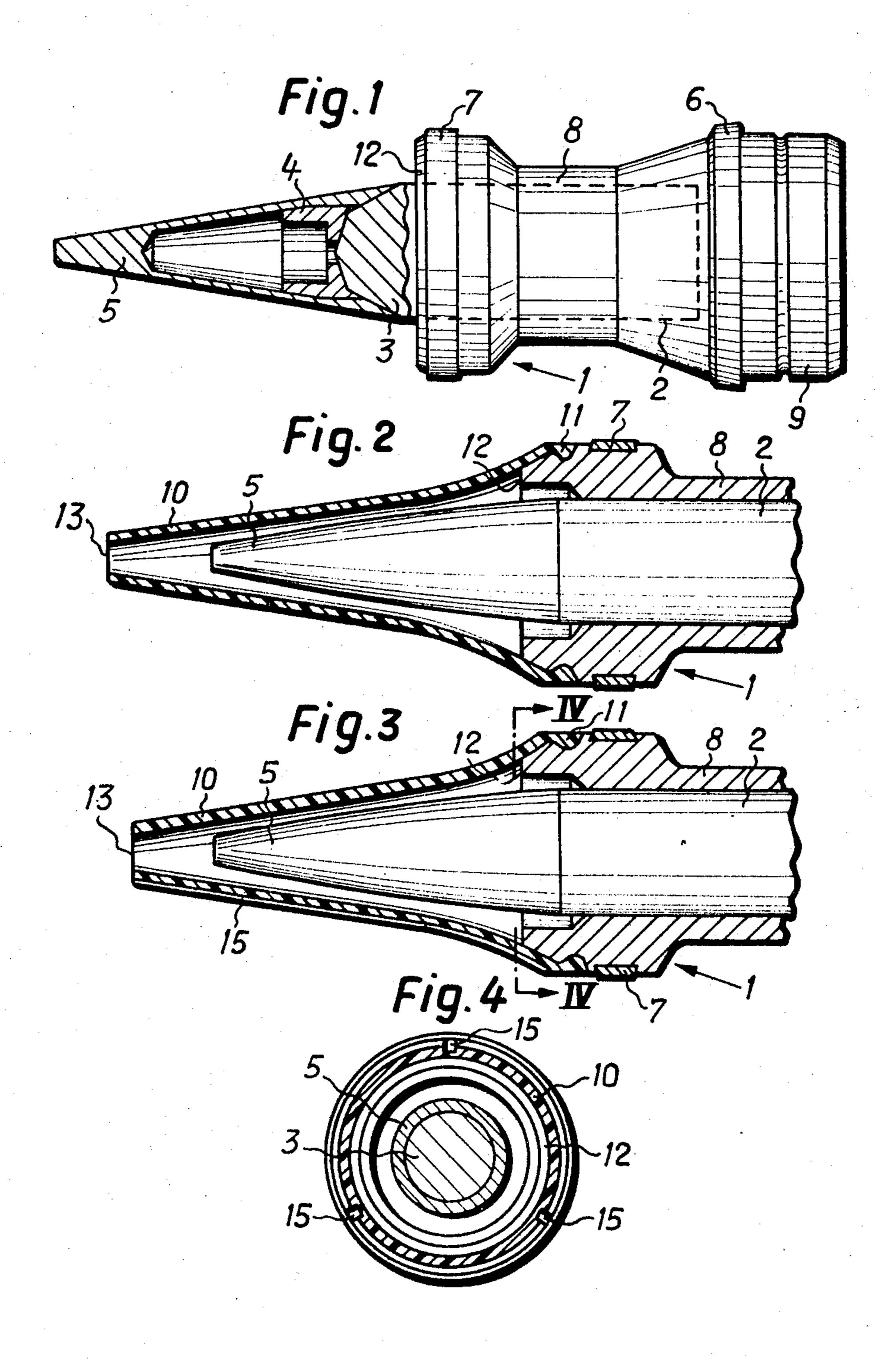
CASING FOR THE SABOT OF A PROJECTILE
