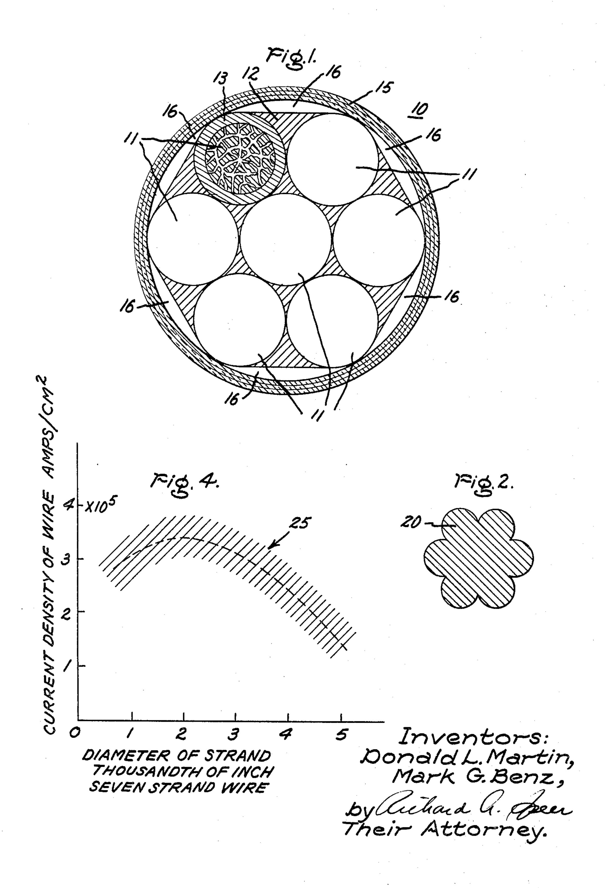
METHOD OF MAKING SUPERCONDUCTORS CONTAINING FLUX TRAPS
