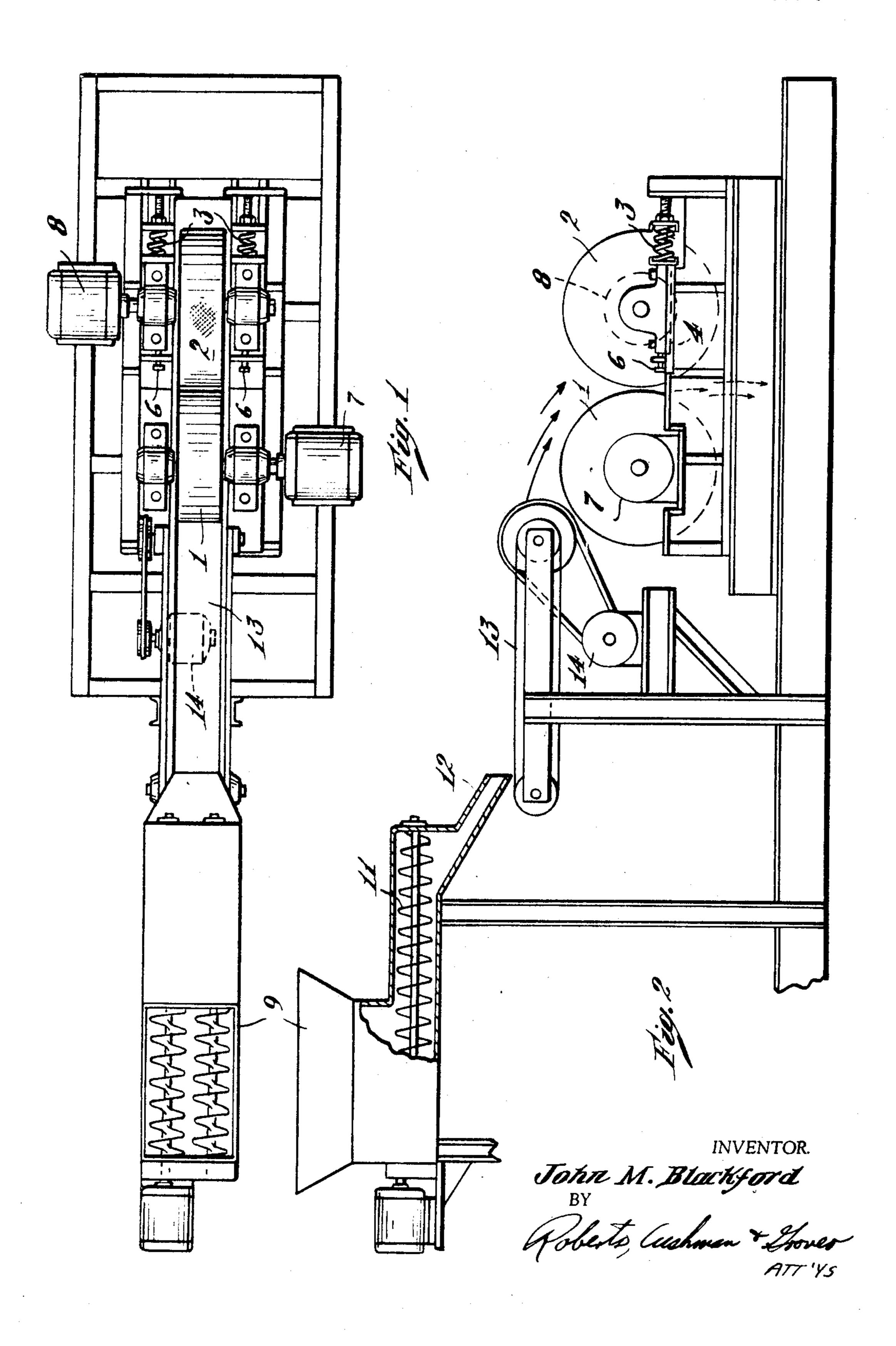
METHOD AND APPARATUS FOR LOOSENING FIBERS OF WOOD CHIPS
