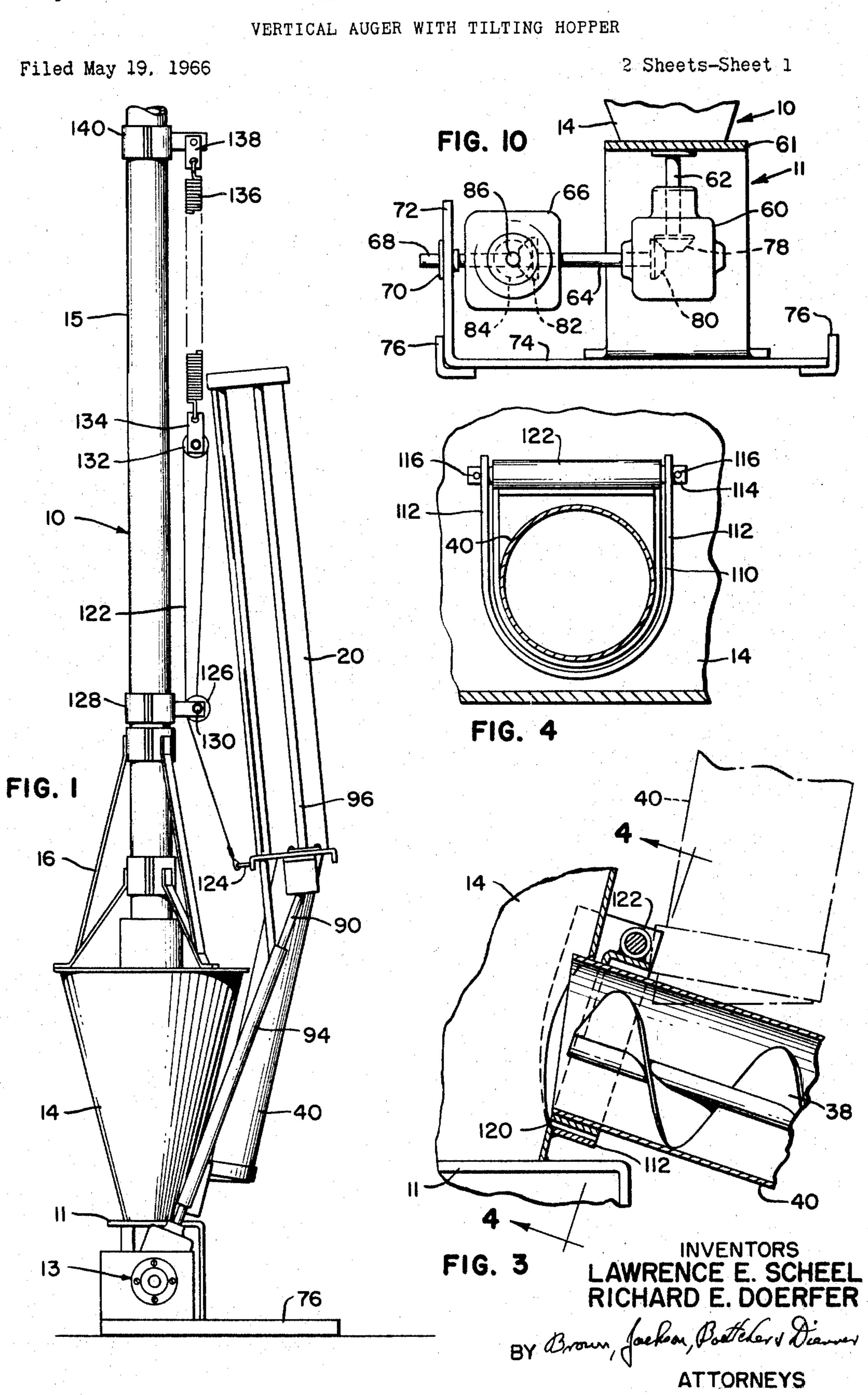
VERTICAL AUGER WITH TILTING HOPPER
