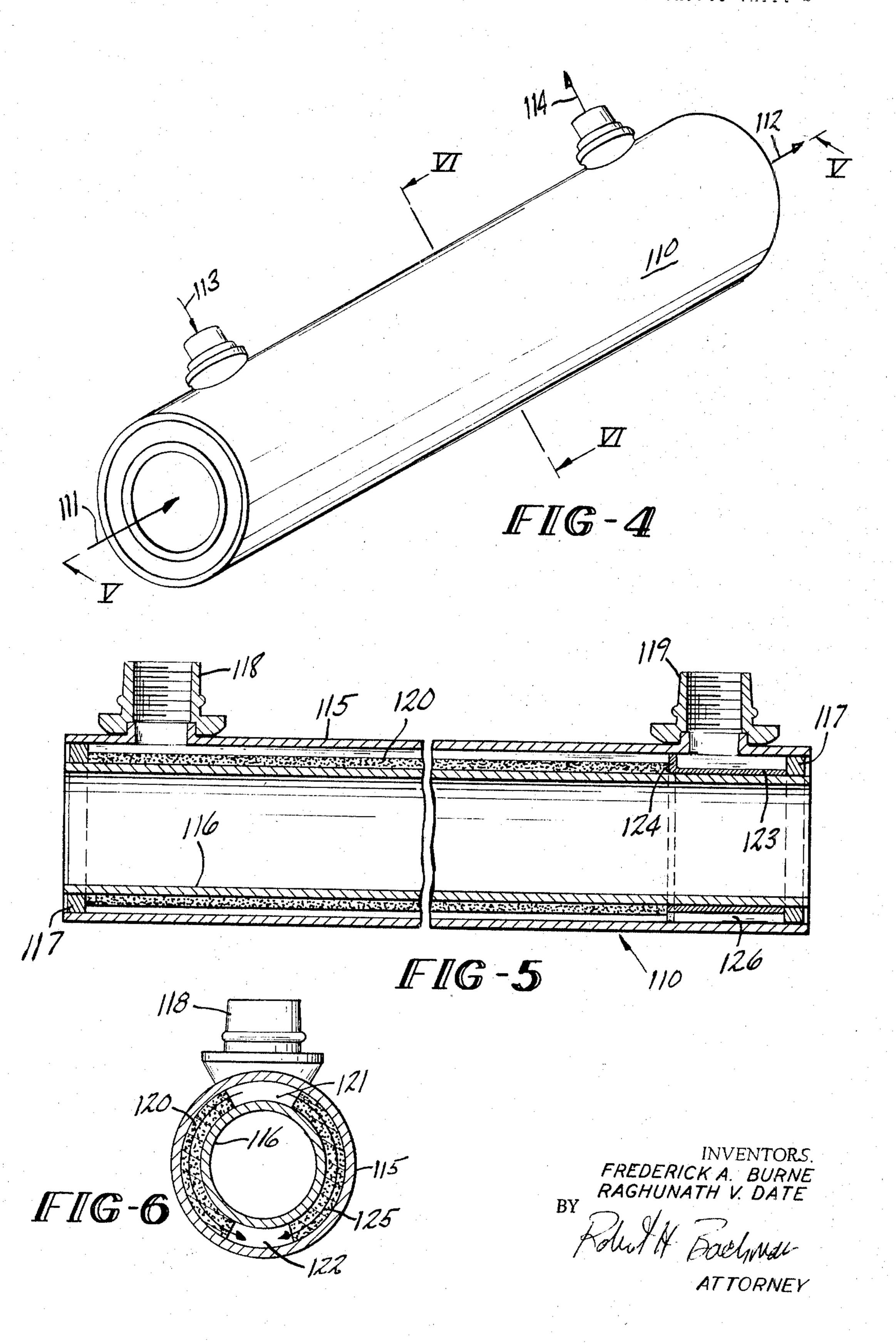
CONCENTRIC TUBE HEAT EXCHANGER WITH SINTERED METAL MATRIX
