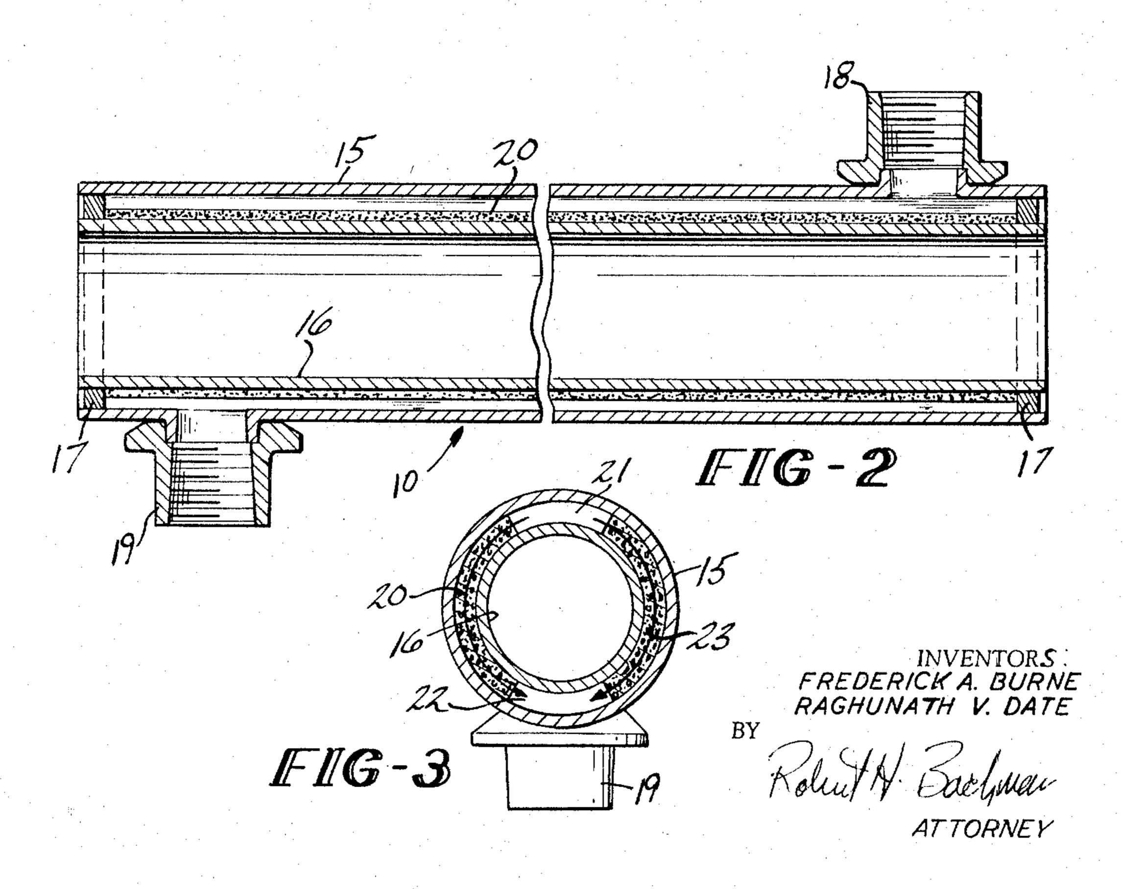
CONCENTRIC TUBE HEAT EXCHANGER WITH SINTERED METAL MATRIX
