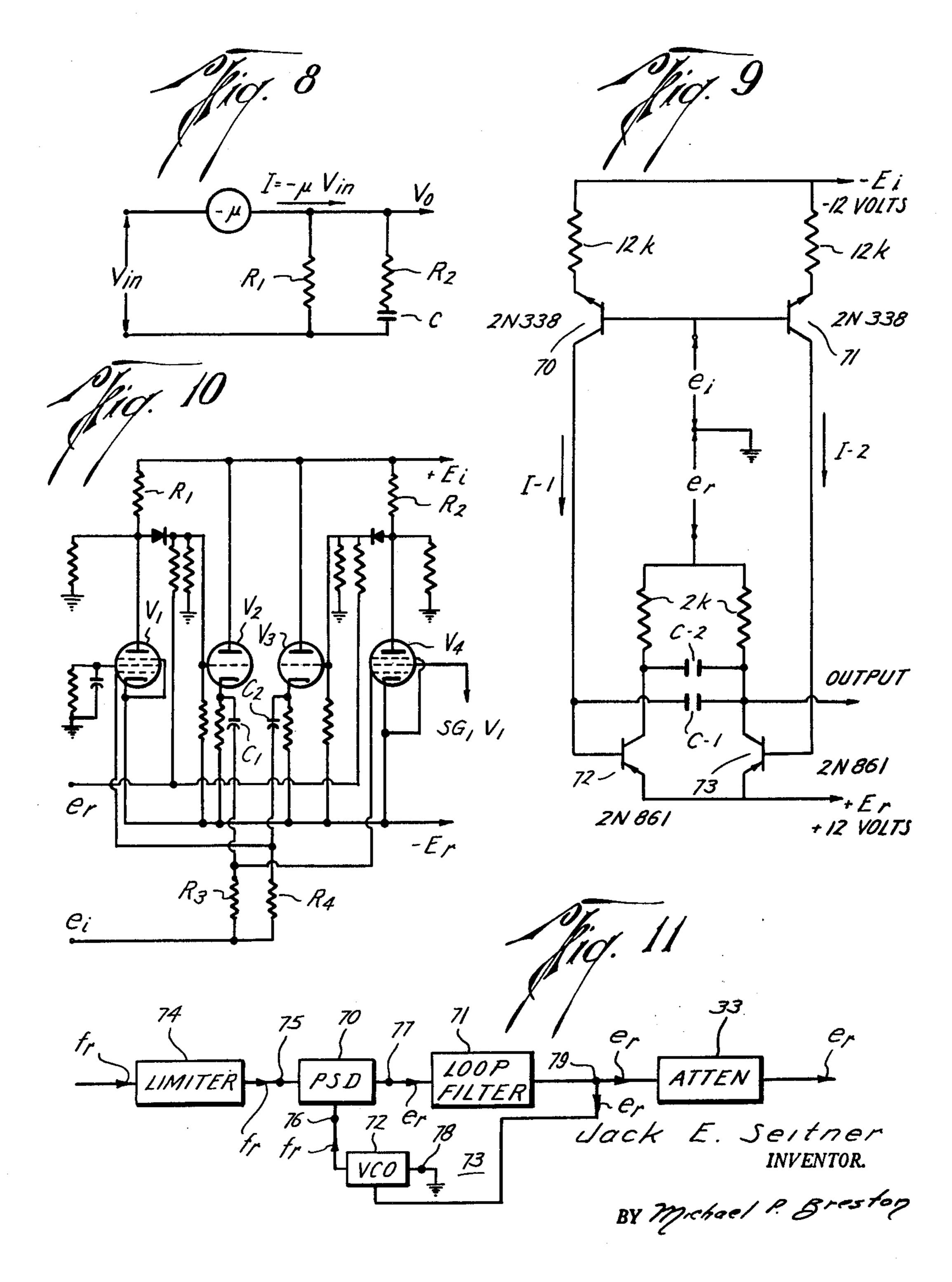
TAPE-SPEED COMPENSATION UTILIZING PHASE-LOCKED LOOP DETECTORS FOR USE IN TELEMETERING SYSTEMS
