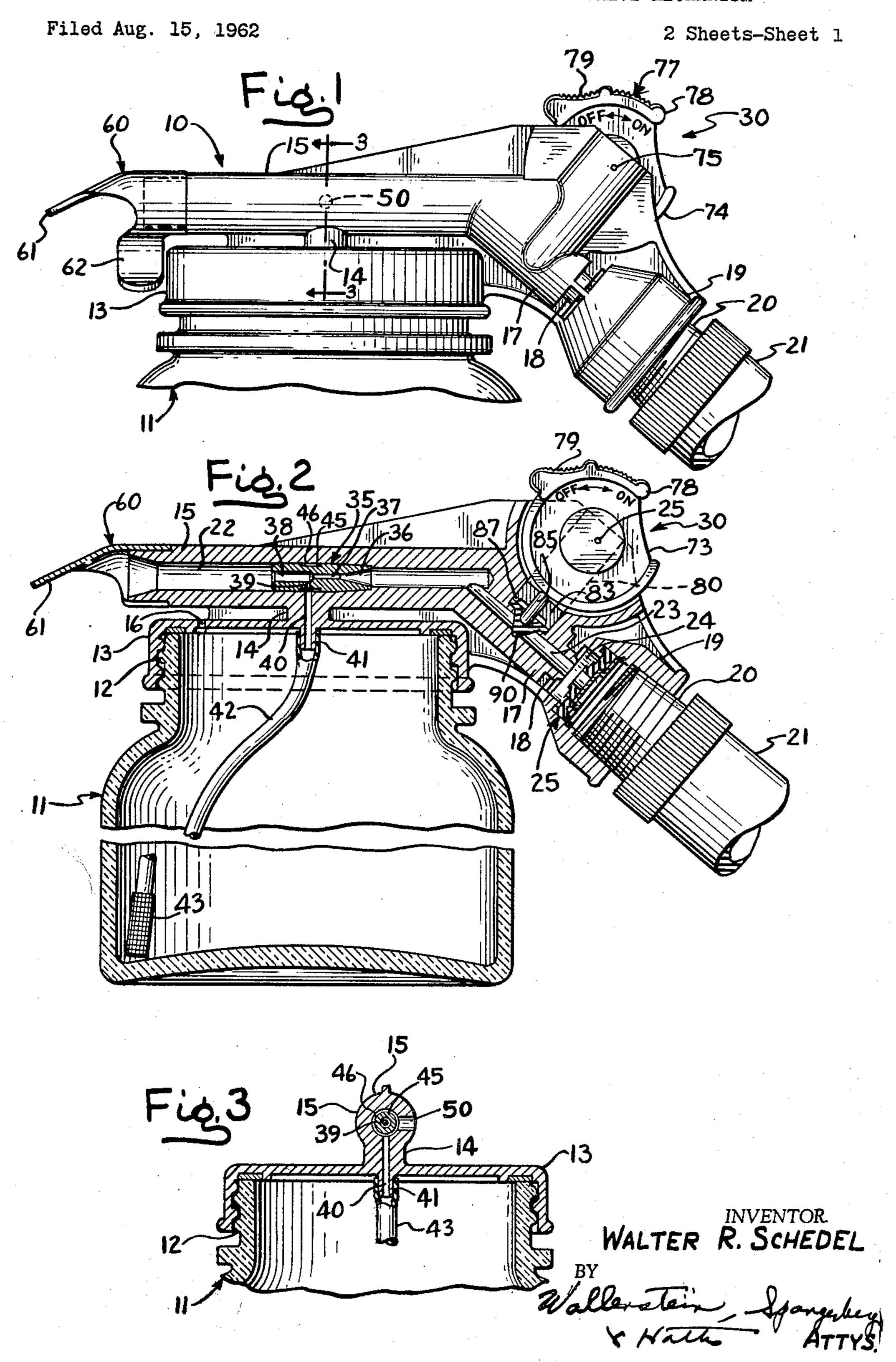
HAND SPRAYER HAVING ON-OFF CONTROL VALVE MECHANISM
