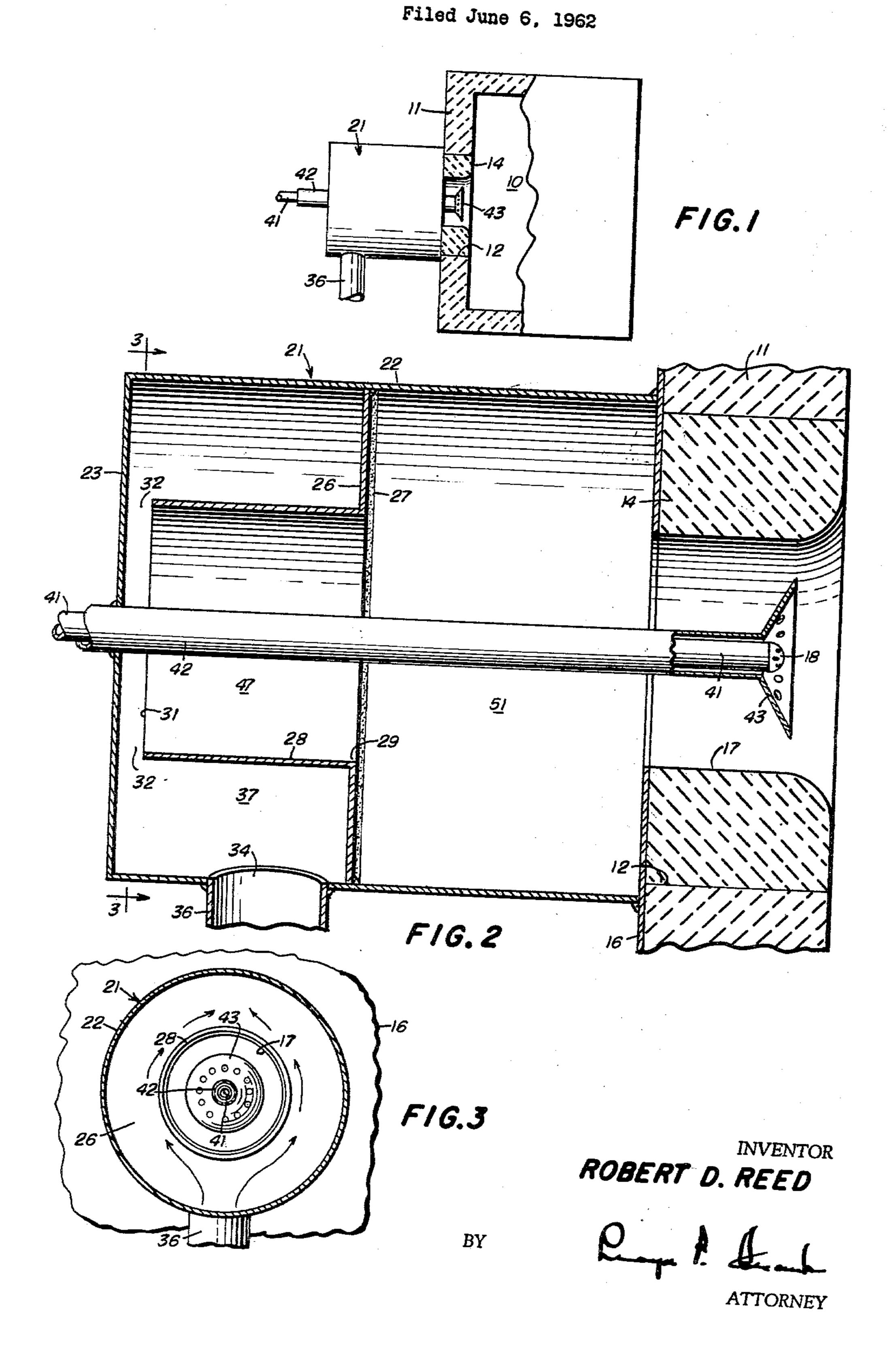
3,180,393 APPARATUS FOR SUPPLYING AIR TO FUEL BURNER
