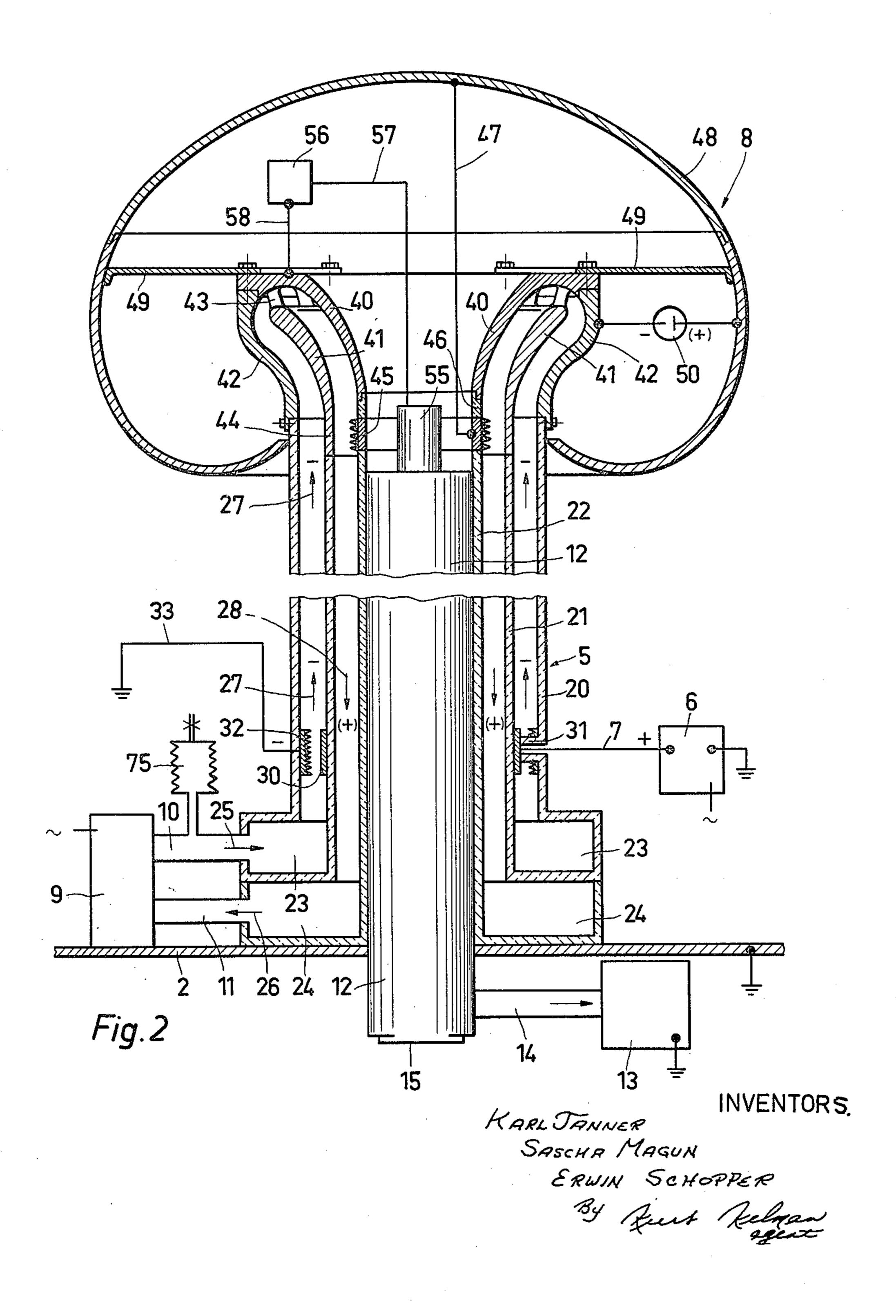
COMBINED ACCELERATOR AND STATIC VOLTAGE GENERATOR
