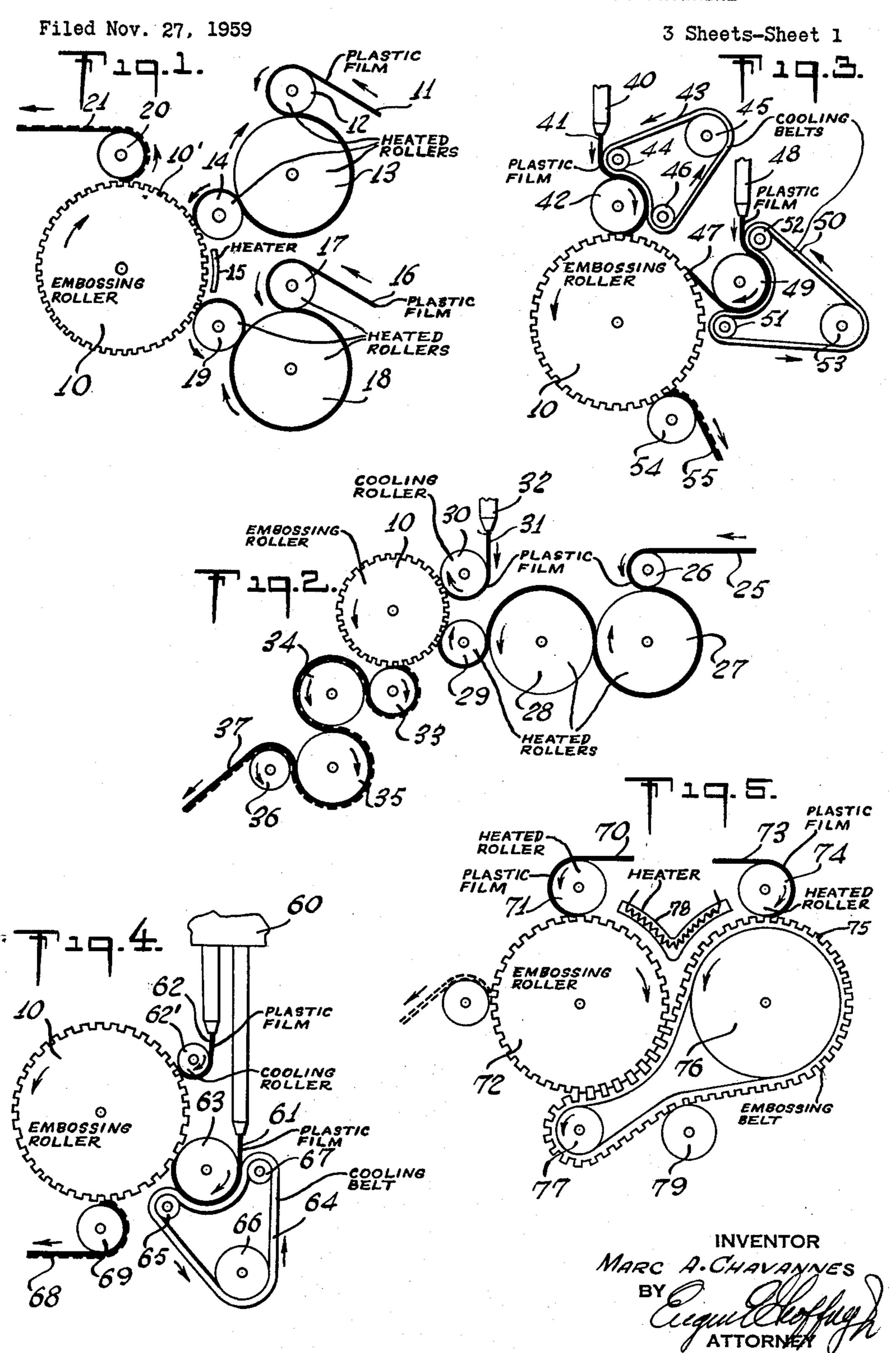
METHOD FOR MAKING LAMINATED CUSHIONING MATERIAL
