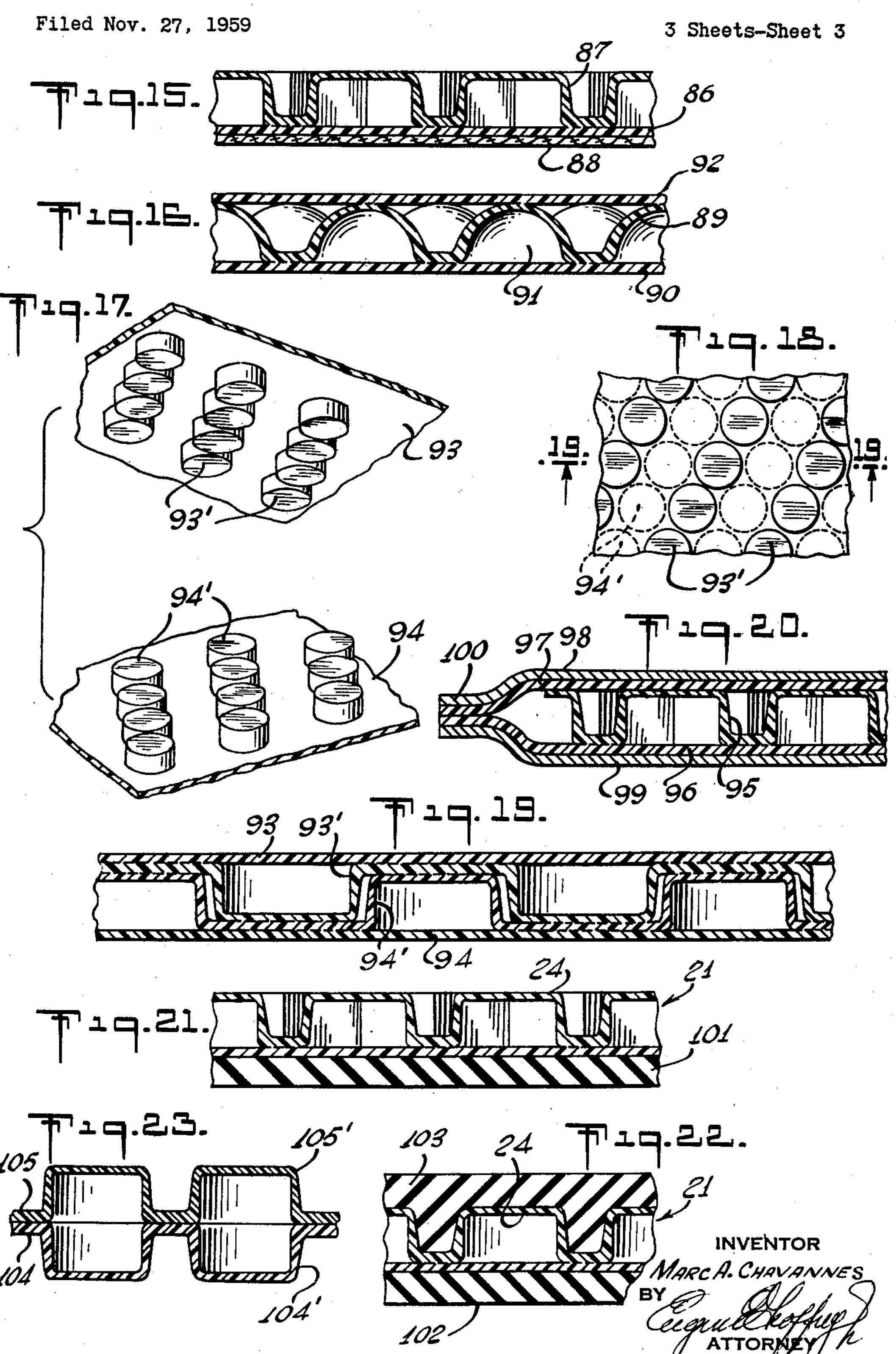
3,142,599 METHOD FOR MAKING LAMINATED CUSHIONING MATERIAL
