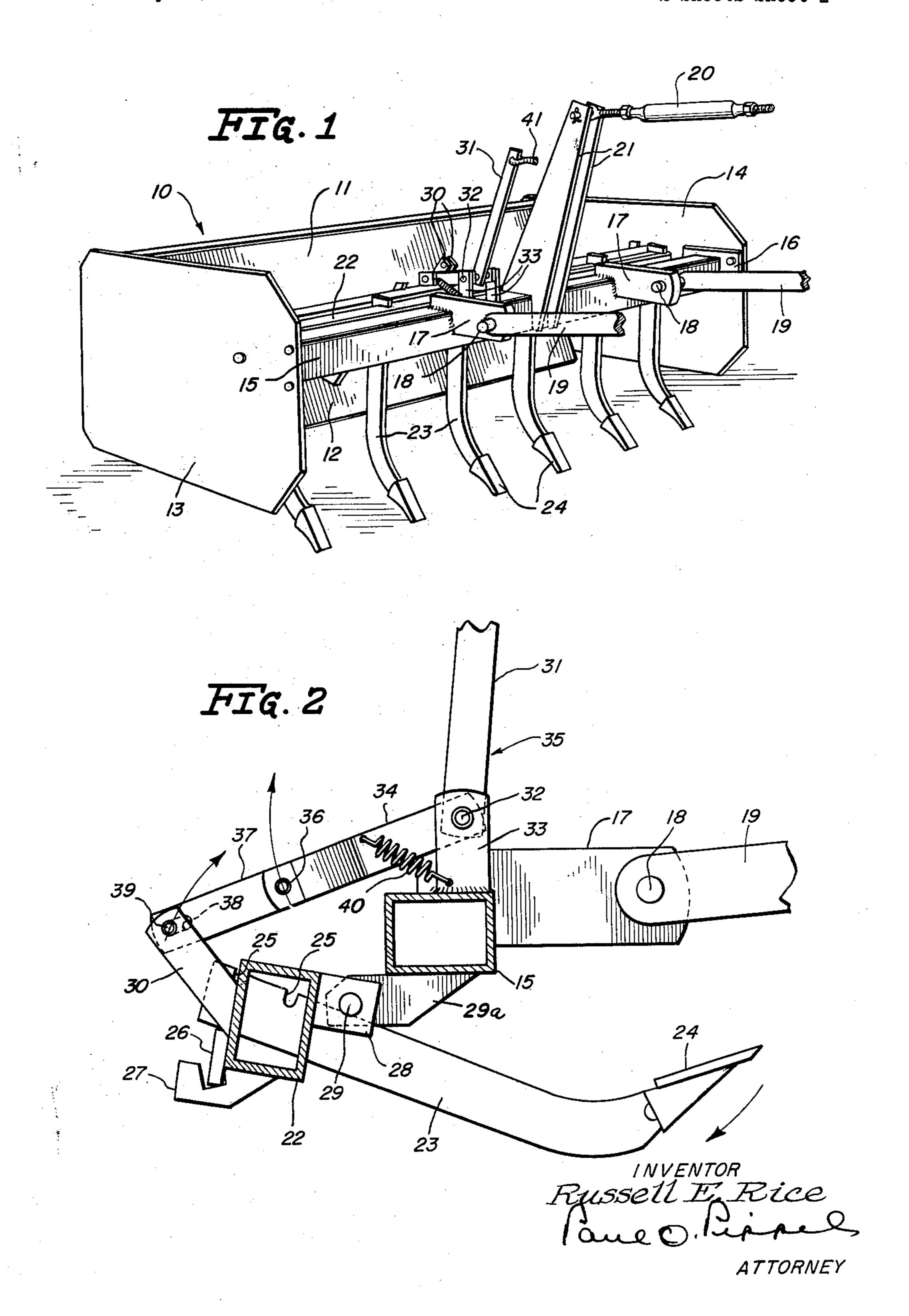
SCARIFIER BAR LOCK MECHANISM
