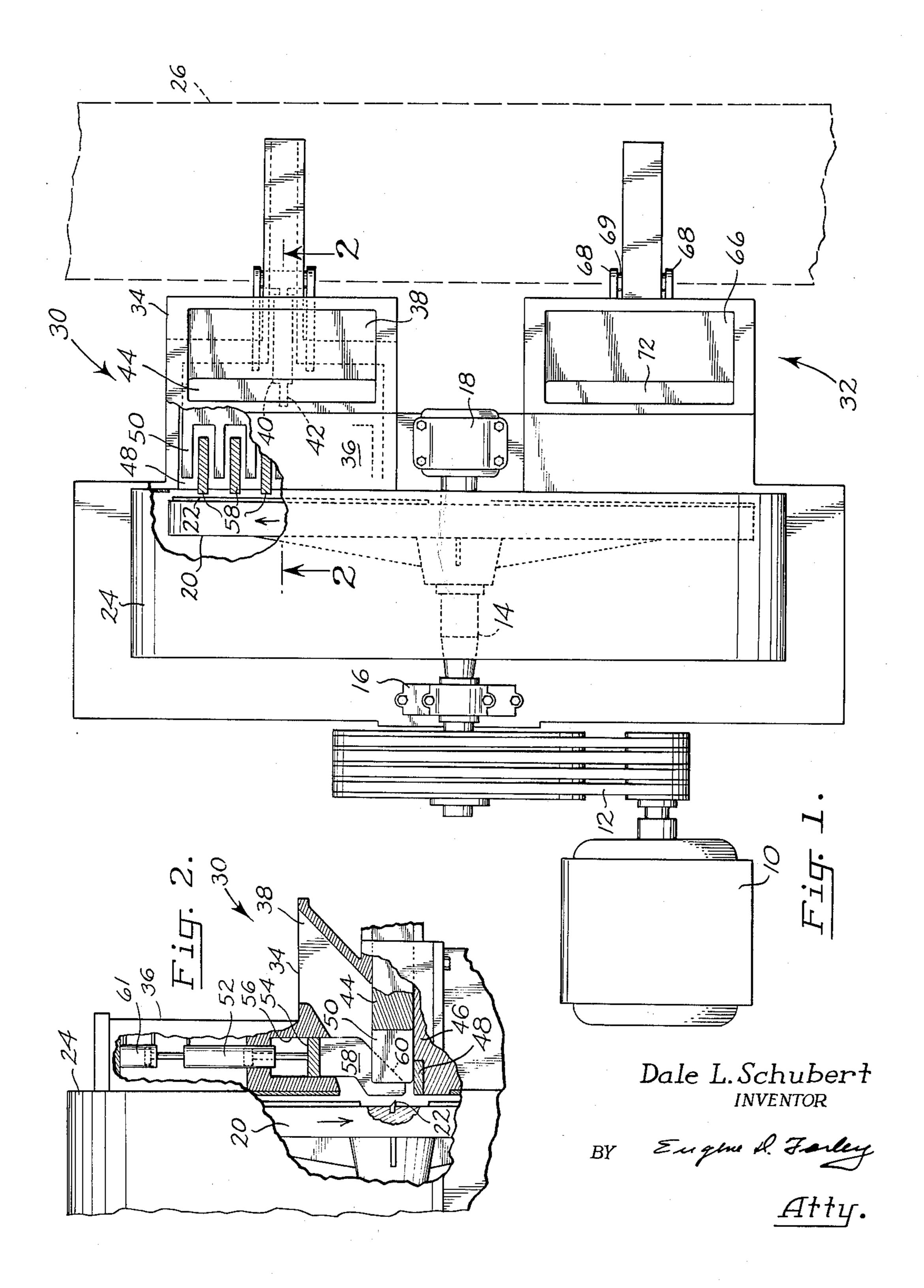
DISC-TYPE WOOD REDUCER WITH MULTIPLE FEED
