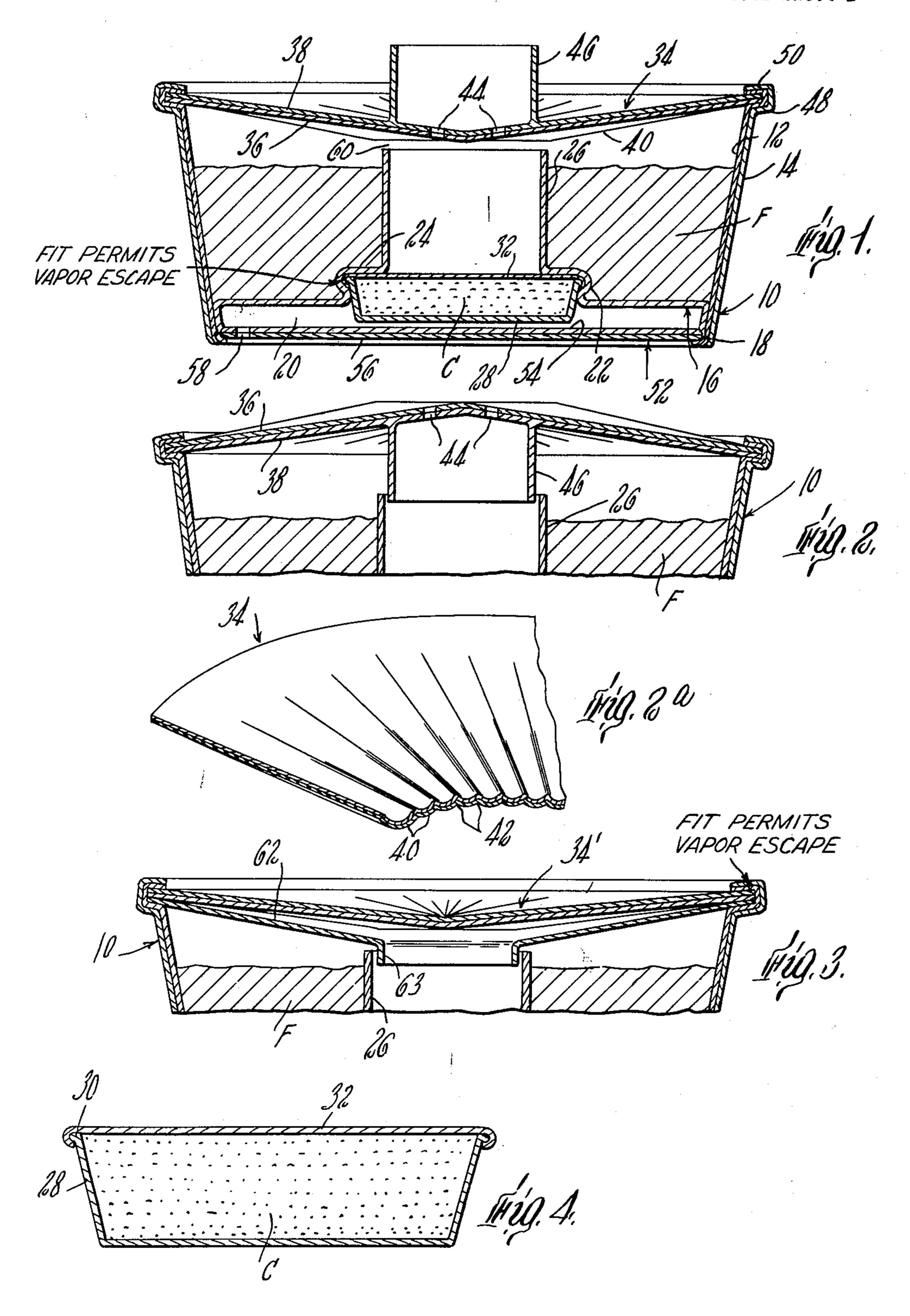
FOOD HEATING DEVICES Filed Feb. 18, 1960 2 Sheets-Sheet 2 FIT PERMITS VAPOR ESCAPE FIT PERMITS VAPOR ESCAPE.
