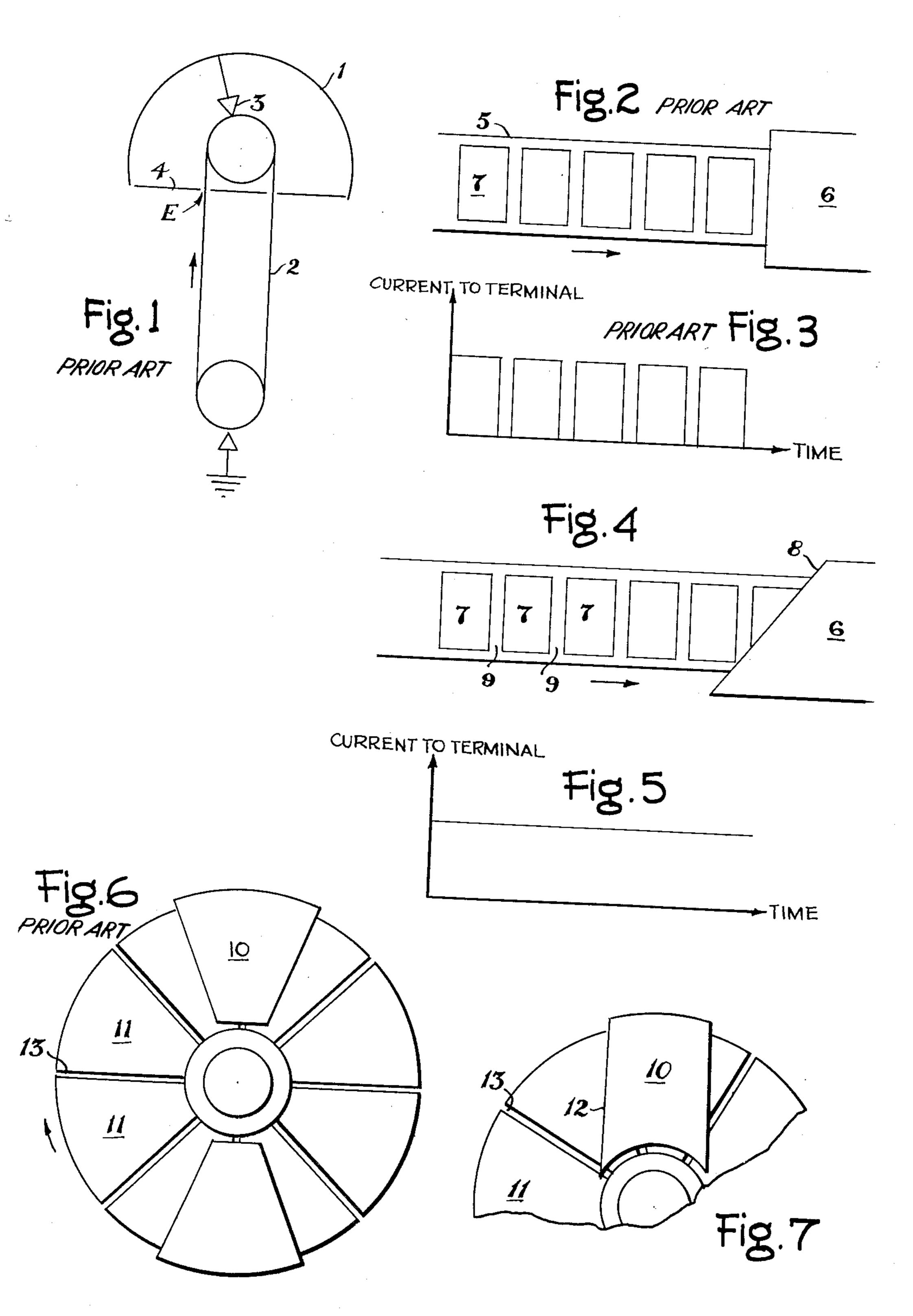
3,056,052 REDUCTION OF VOLTAGE FLUCTUATIONS IN ELECTROSTATIC EQUIPMENT
