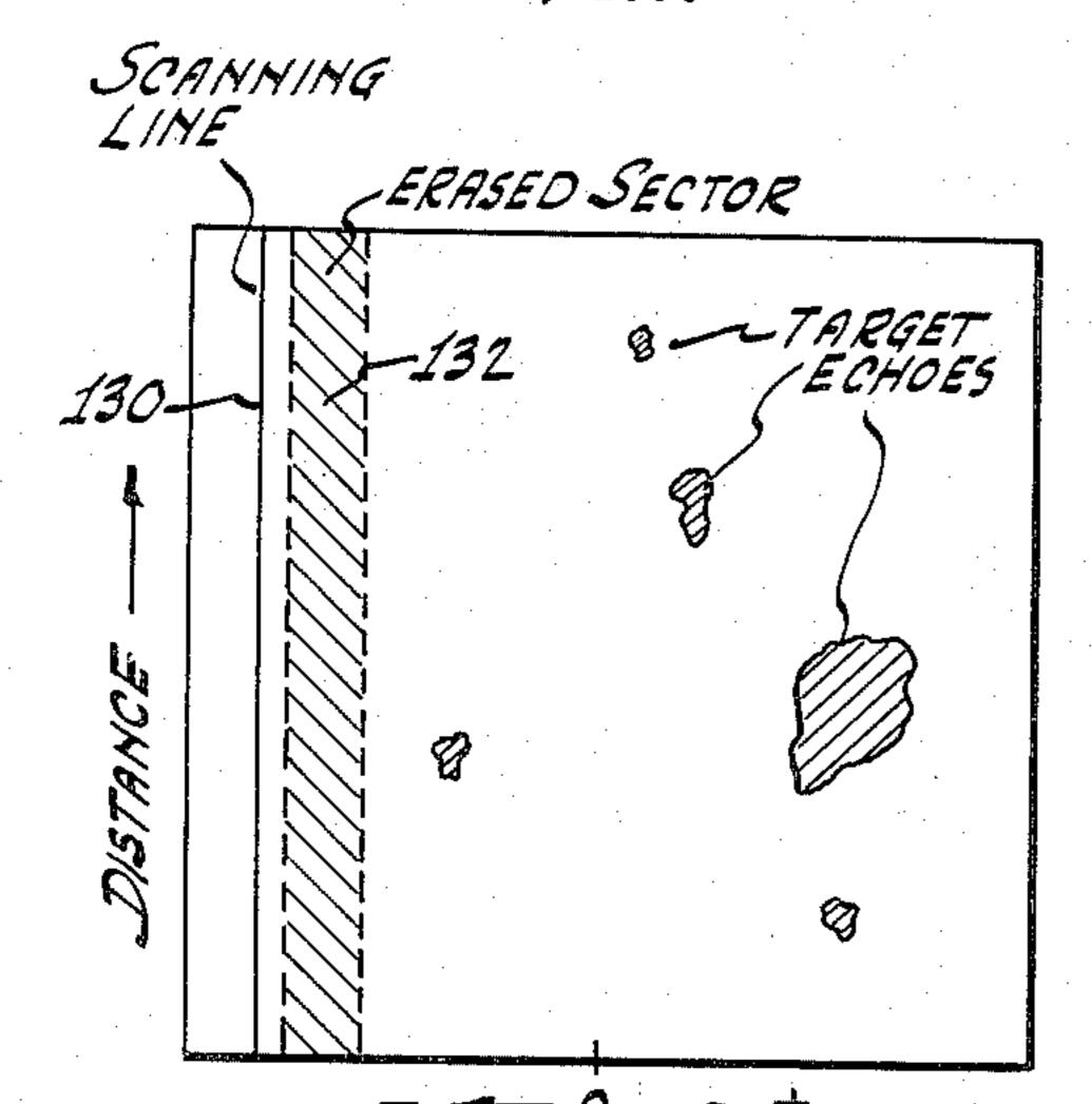
AZIMUTH ANGLE \_ DIRECTION OF MOVEMENT OF SCANNING LINE Fig. 50.
