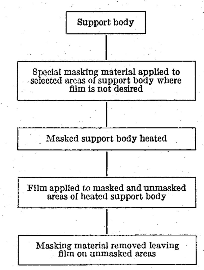
It is accordingly a primary object of this invention to provide a novel technique for preventing the formation of electrically conducting film on unwanted areas of a filmed base that is simpler, faster and more economical than the procedures heretofore available.
