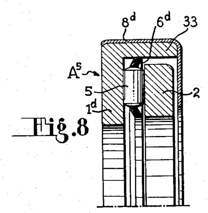
CLUTCH THRUST BEARING AND DEVICE EQUIPPED WITH THE LATTER
