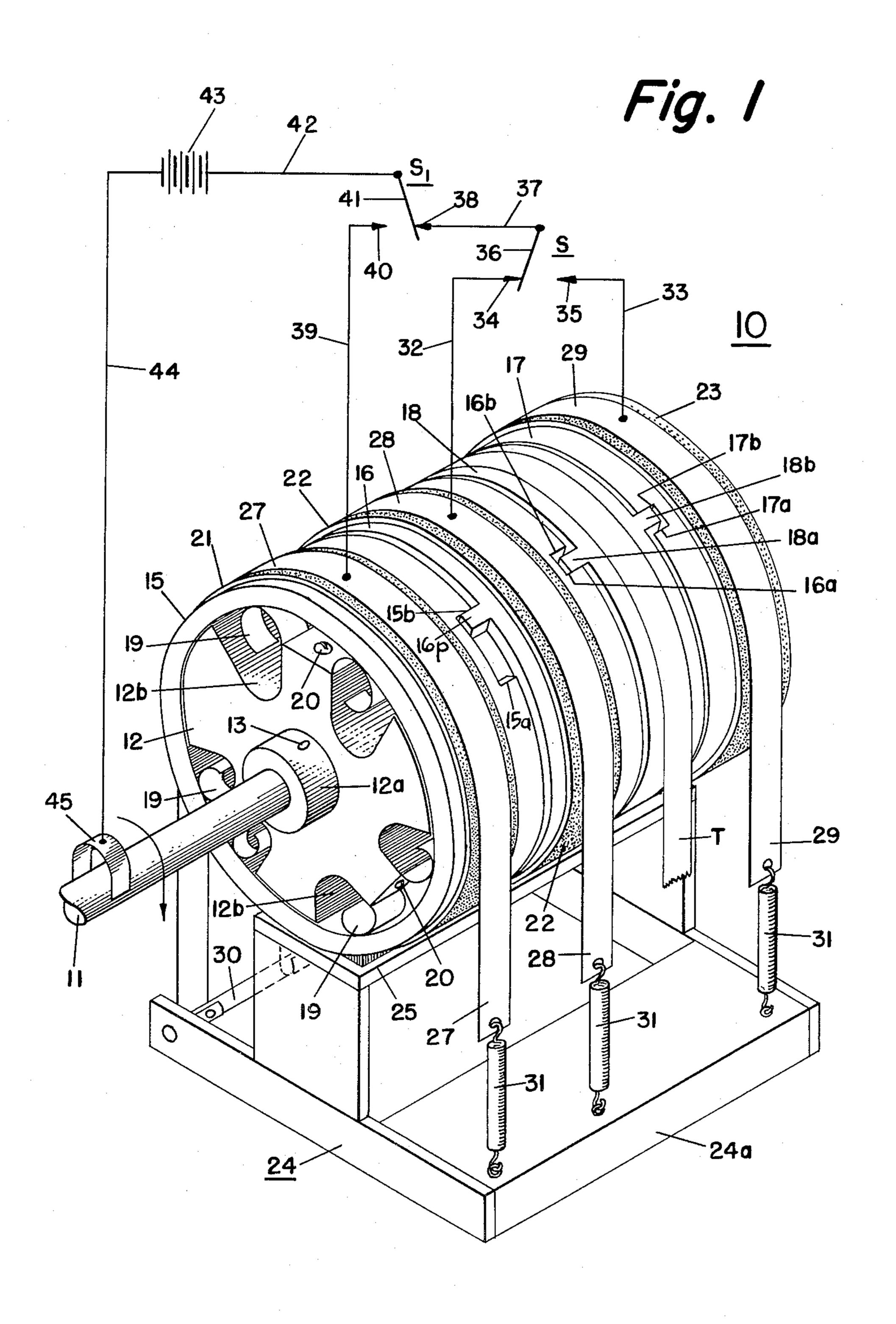
ELECTROSTATIC INCREMENTAL DRIVE UNIT
