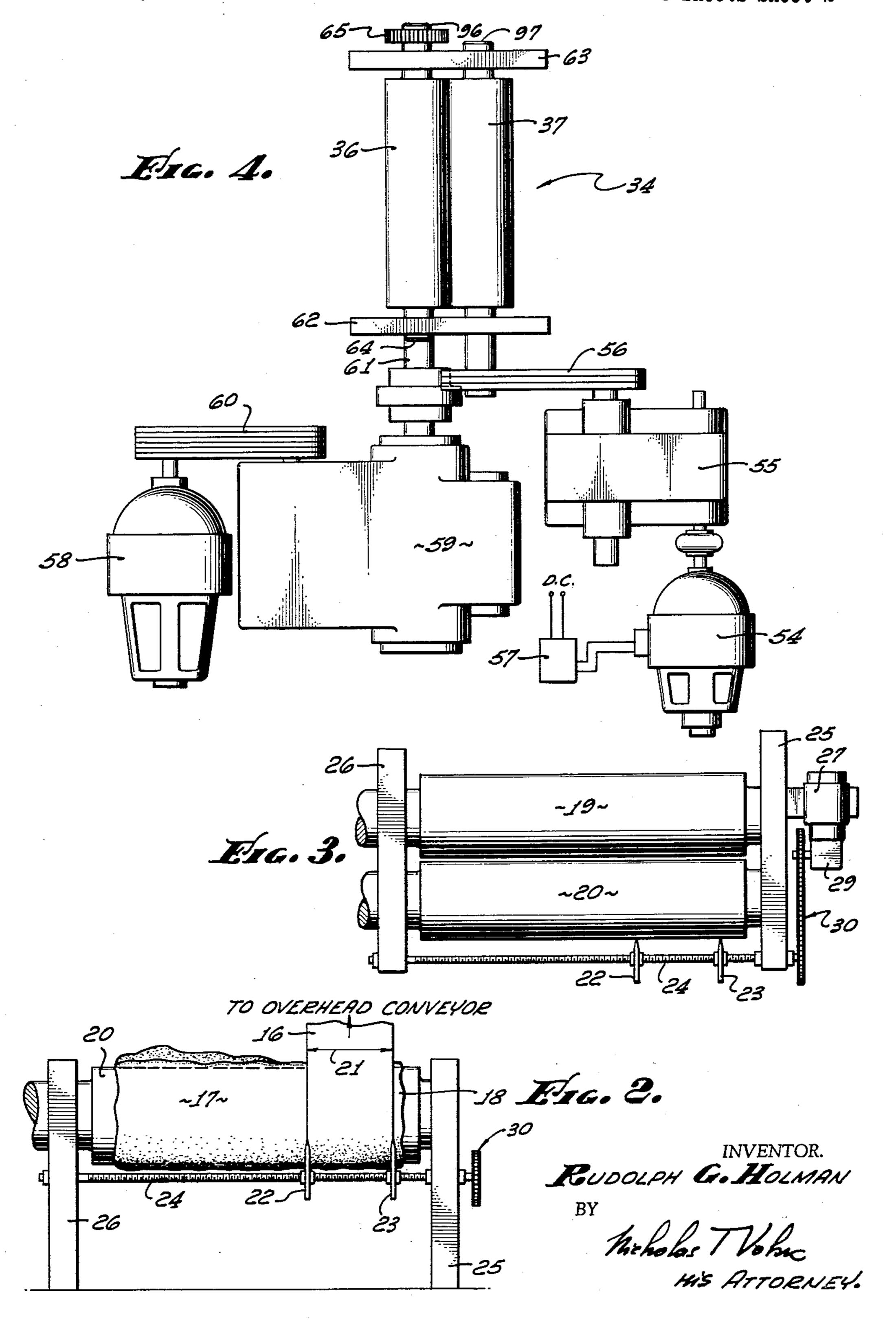
APPARATUS FOR PRODUCING A CONTINUOUS STRIP OF ELASTIC MATERIAL
