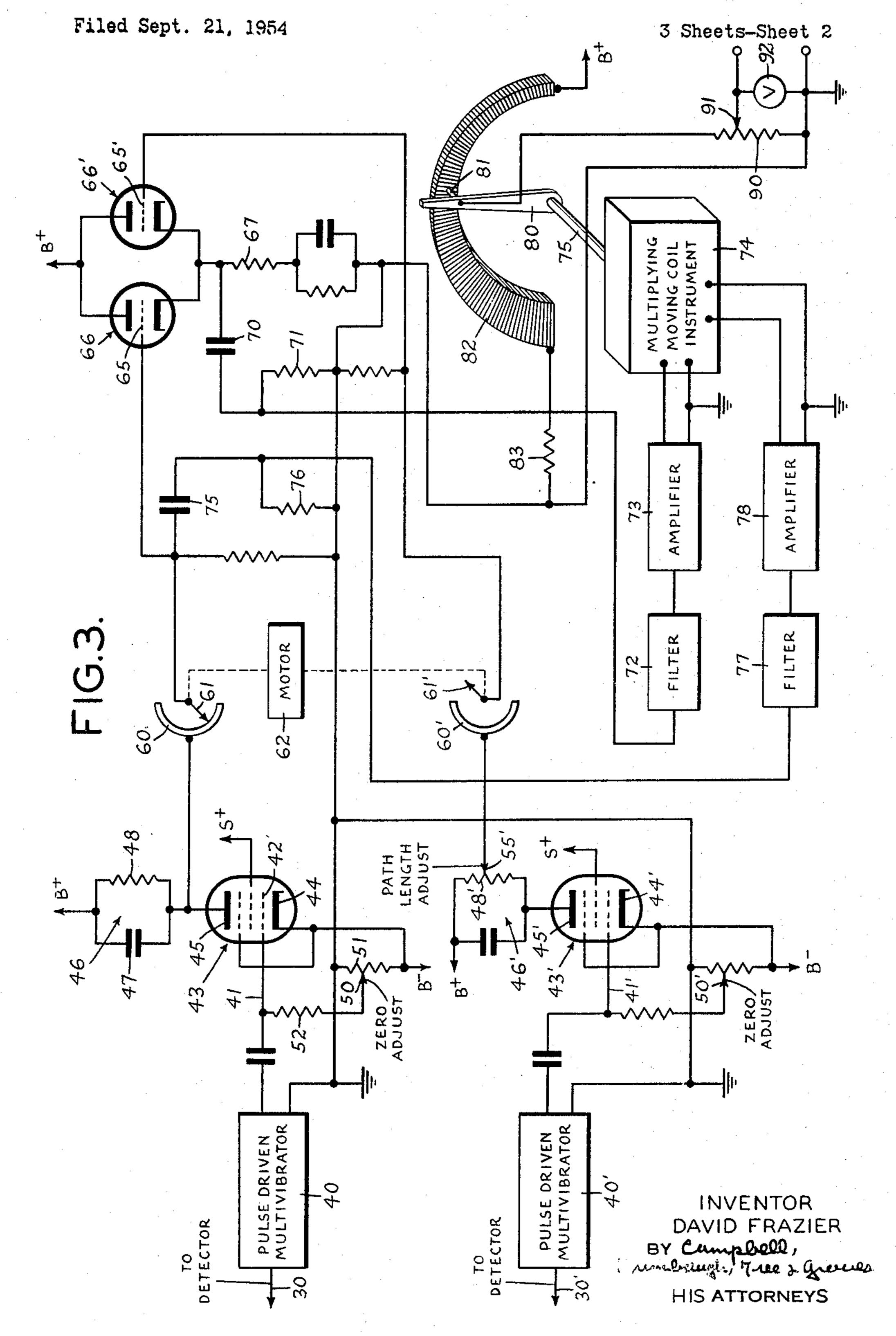
SYSTEM FOR MEASURING MASS FLOW RATE BY RADIATION
