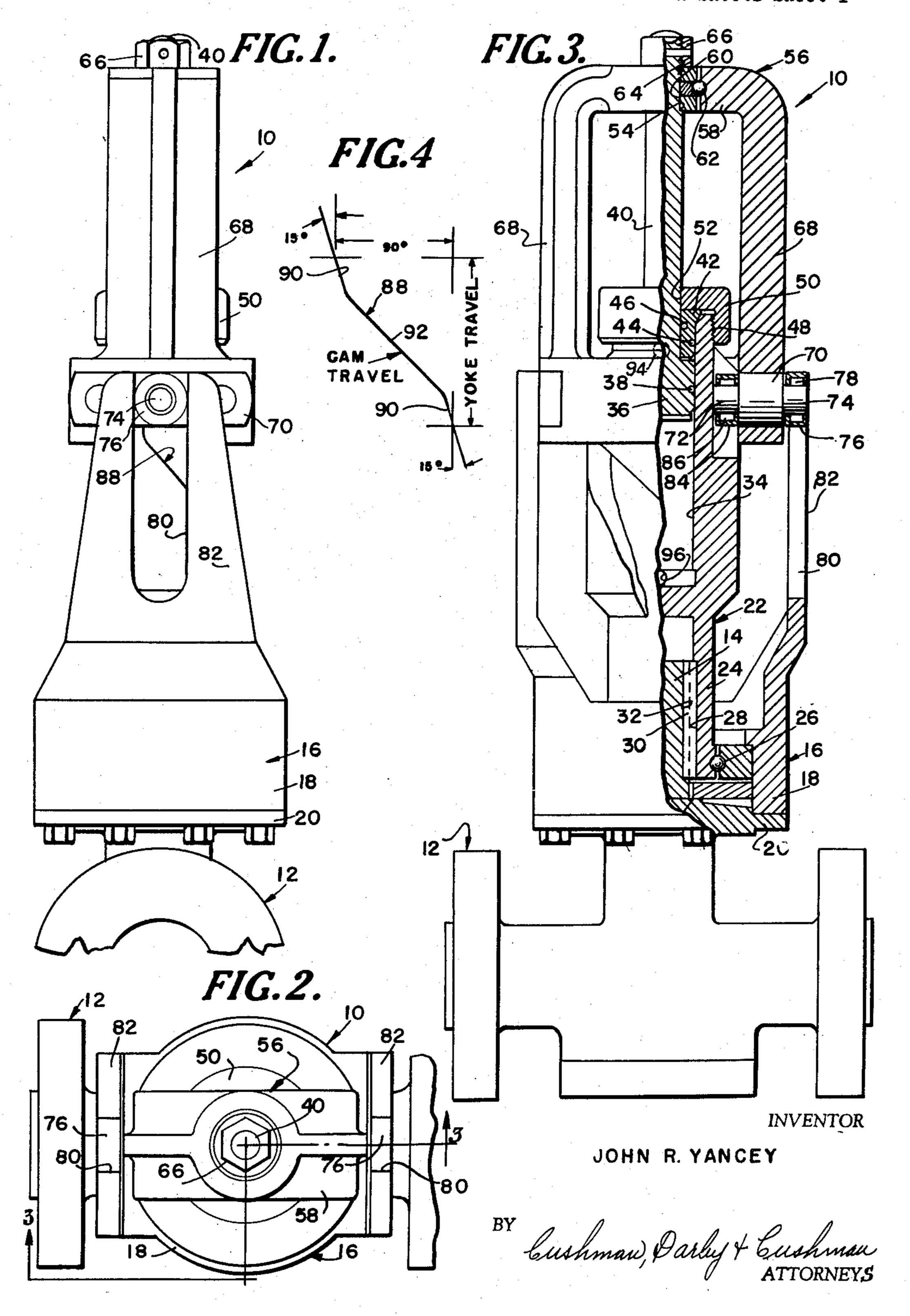
VALVE ACTUATING MECHANISM
