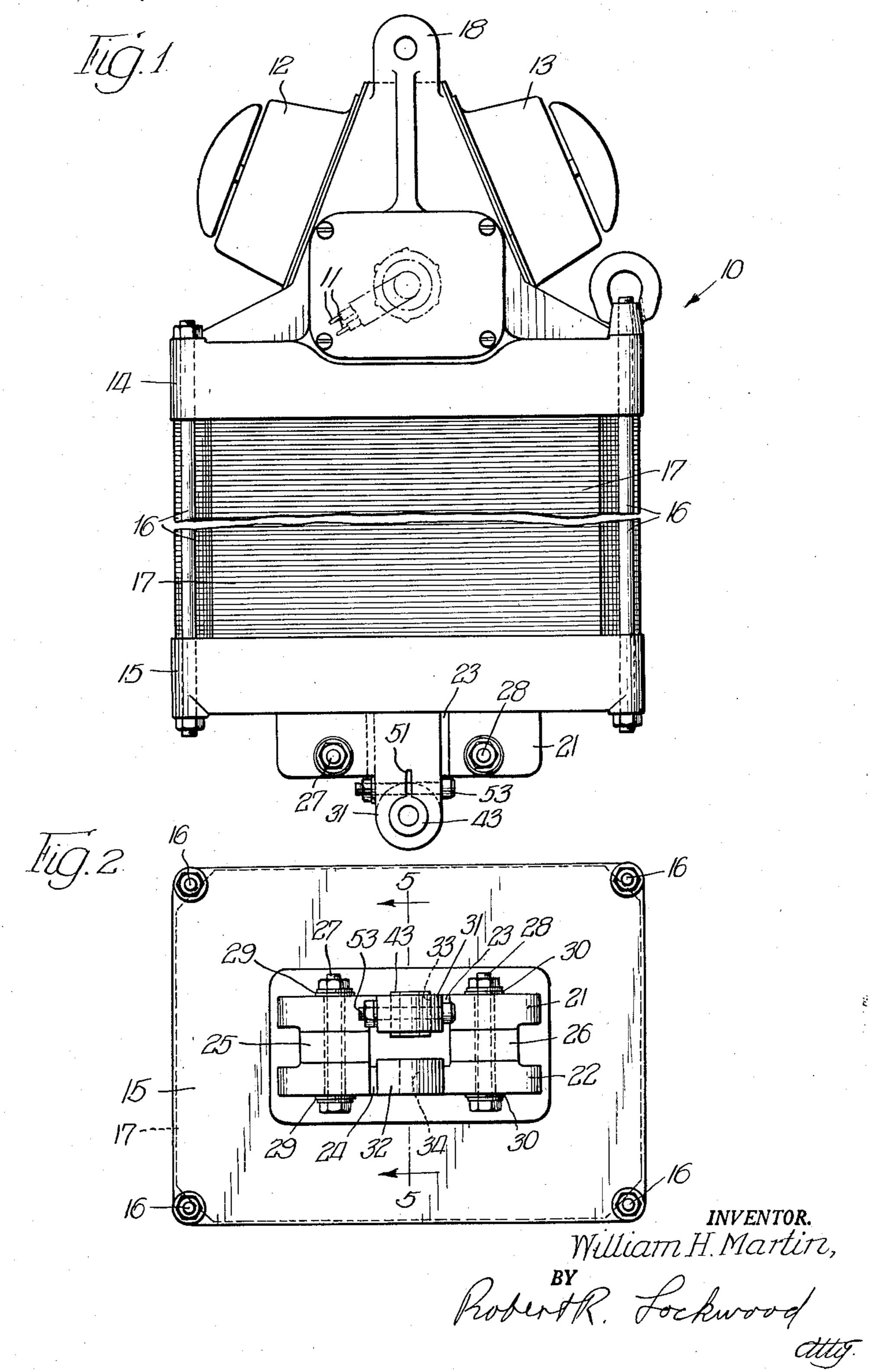
CONNECTING MEANS FOR WELDING CABLE AND TRANSFORMER
