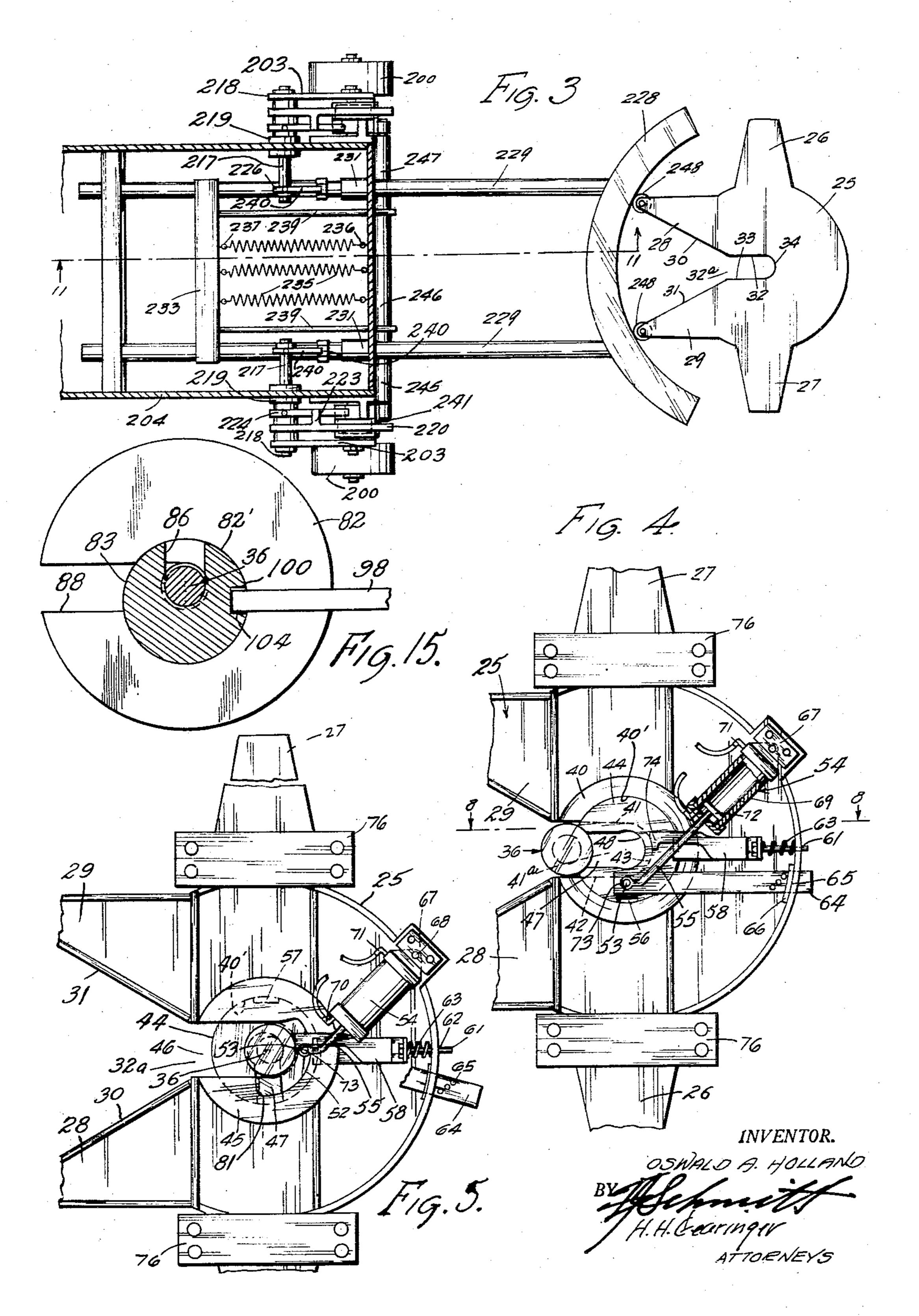
FIFTH WHEEL HAVING A REMOTE CONTROLLED LOCKING MECHANISM
