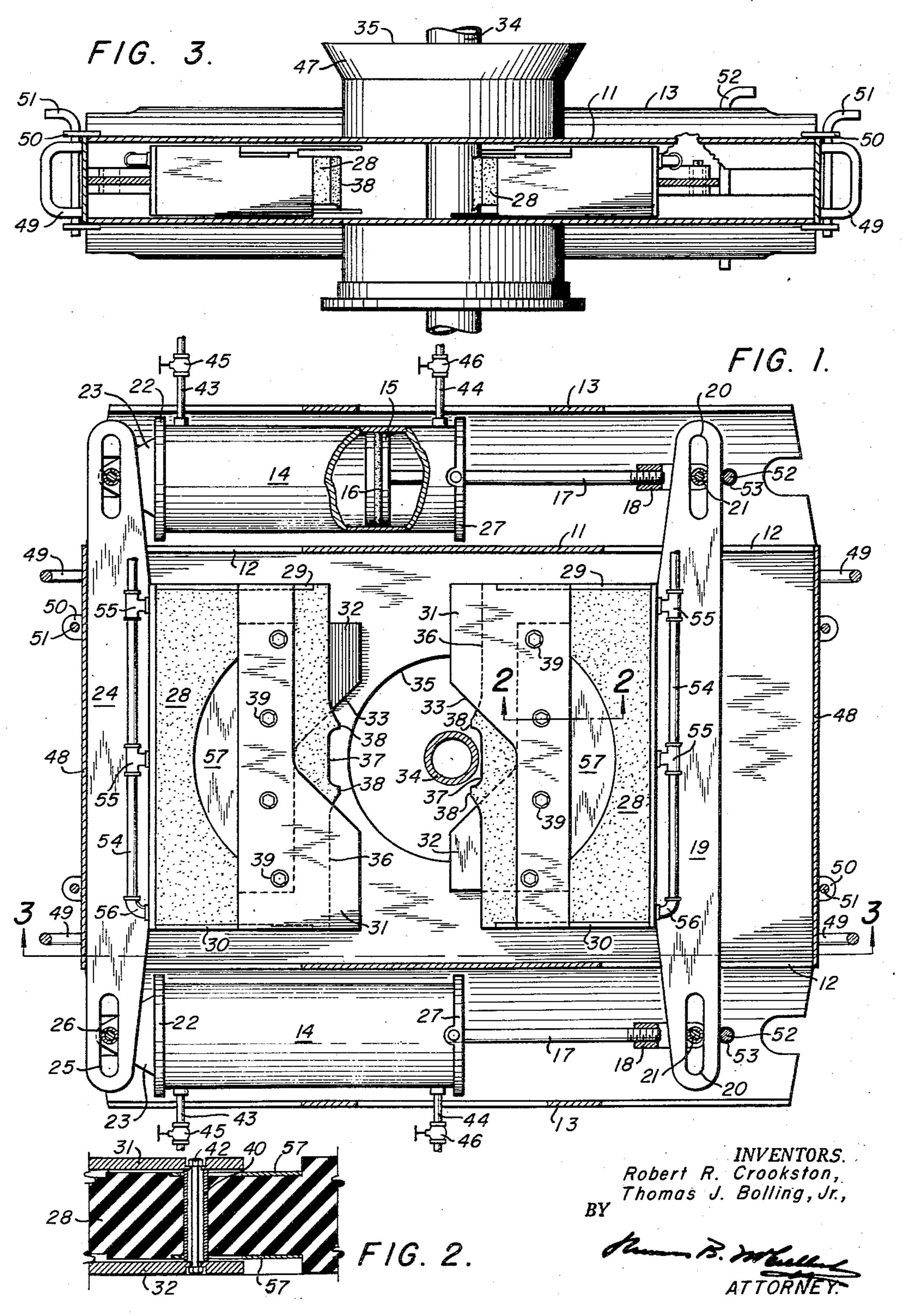
LATERALLY ADJUSTABLE BLOWOUT PREVENTER WITH INFLATABLE RAMS
