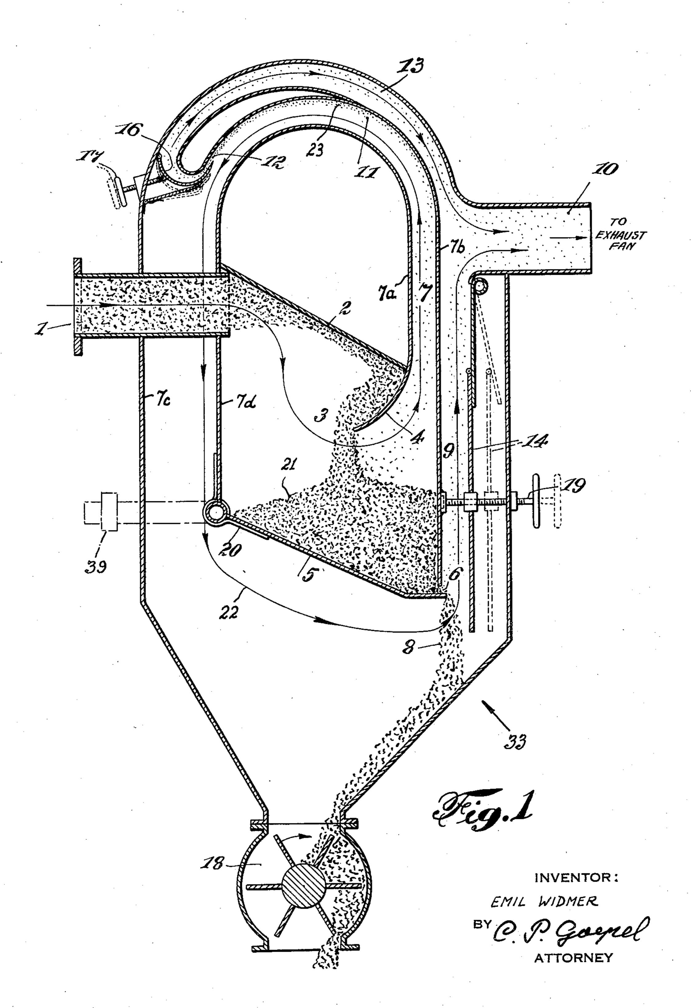
SEPARATORS FOR PNEUMATICALLY CONVEYED AGGREGATE GOODS
