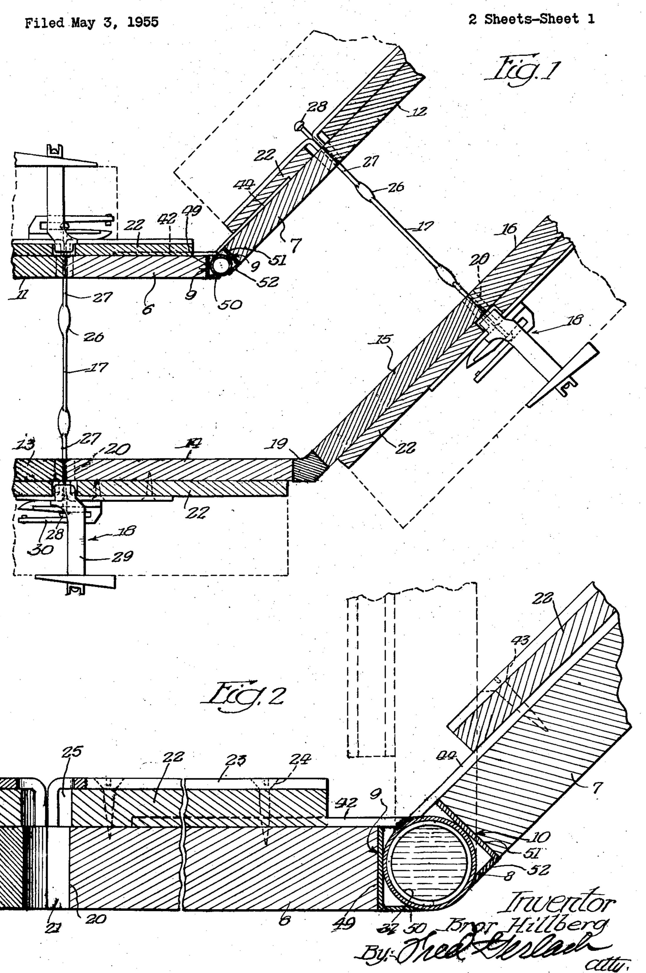
INNER CORNER FORMING UNIT FOR A CONCRETE WALL FORM
